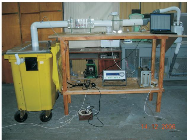
**Fig. 2.** Laboratory unit with the fermentation chamber as inventory gases source and gas analyzer for evaluation filter with granular filler working.
