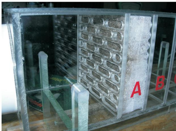
**Fig. 1.** Filtration layer during the experiment – blanching of filler visible.
