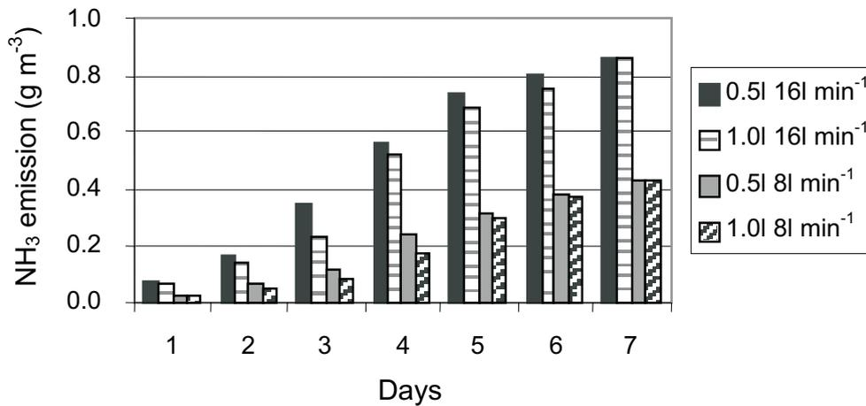
Fig. 4. NH<sub>3</sub> emissions for airflow rates 8 and 16 l min<sup>-1</sup> after application of 0.5 and 1 l of filtration filler, respectively.
