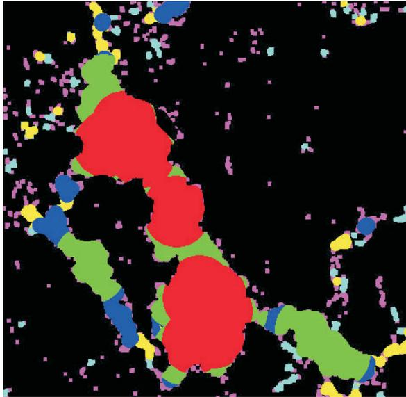
**Fig. 6.** Macropores divided into six fractions according to pore diameter. (>2000  $\mu\text{m}$ , red; 1000-2000  $\mu\text{m}$ , green; 500-1000  $\mu\text{m}$ , blue; 200-500  $\mu\text{m}$ , yellow; 100-200  $\mu\text{m}$ , light blue; 50-100  $\mu\text{m}$ , purple color).
