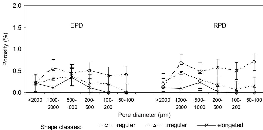
Fig. 10. Pore distribution of compacted soil (D90) according to EPD and RPD. Bars represent standard error.
