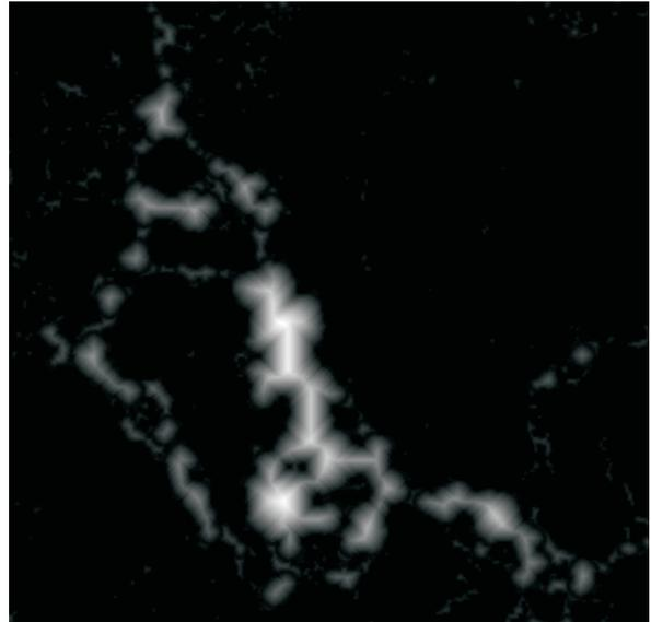
**Fig. 4.** Image after `mgGraphDistance` operator. The brightness of pixels depends on the distance between the centre and the border of objects.
