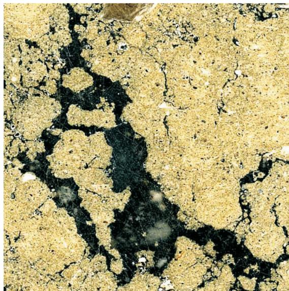
**Fig. 1.** Cross section of soil from 10-18 cm soil layer (fragment with dimensions of 2x2 cm, pores appear black).
