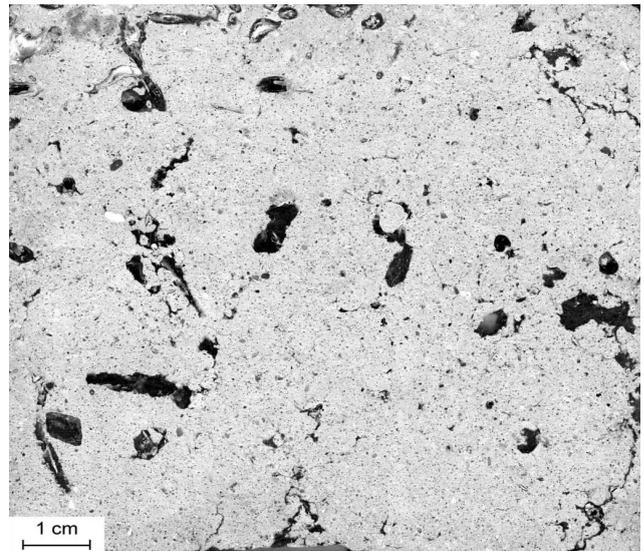
**Fig. 8.** Example of compacted (D90) soil sample (pores appear black).
