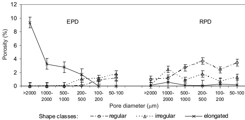
Fig. 9. Pore distribution of porous soil (D70) according to EPD and RPD detection. Bars represent standard error.
