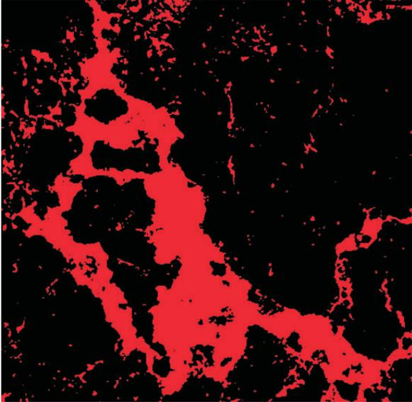
**Fig. 2.** Macropores selected by `ImgMaximumContrastThreshold` operator (pores appear red).
