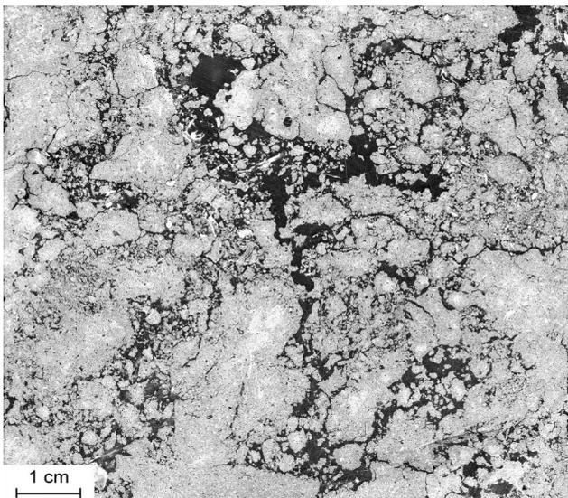
**Fig. 7.** Example of porous (D70) soil sample (pores appear black).
