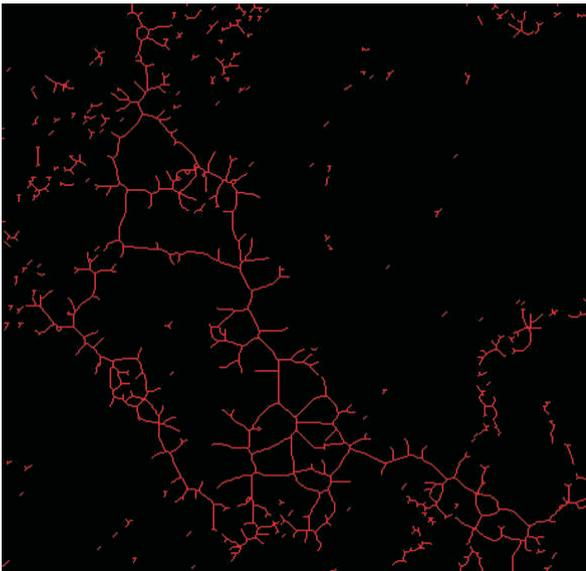
**Fig. 3.** Skeleton of macropores after `ImgThinSkeleton` operator.
