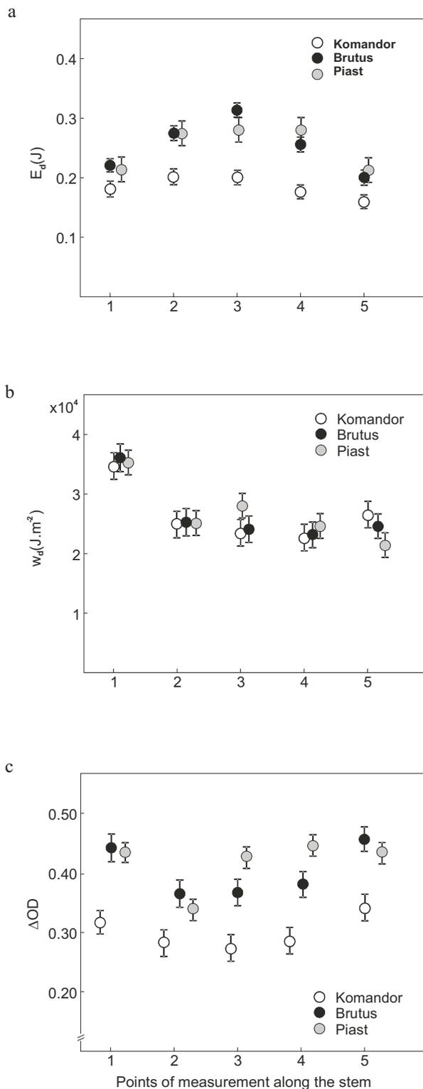
**Fig. 1.** Mean values and 95% Tukey HSD intervals: a – of the cutting work ( $E_d$ ), b – of the cutting work per stem total cross-section area ( $w_d$ ), and c – of the value of  $\Delta OD$ ; for experimental points on the length of pea stems (1..5 points on the length of stems from the root to the tip, for complete pod filling and full ripeness).
