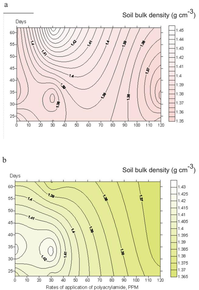
**Fig. 2.** Relationships between rates of application of polyacrylamide (PPM), the time since the start of experiment (days), and soil bulk densities for special case when wheat residue is: a – not incorporated in soil (none), b – incorporated in soil (wheat residue added).
