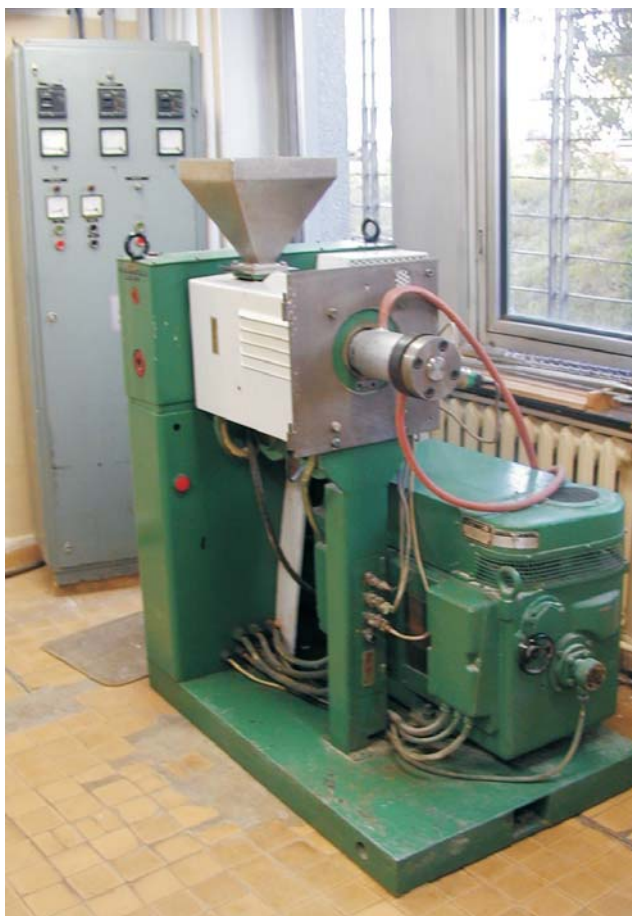
Fig. 1. Modified single screw extruder TS-45.
