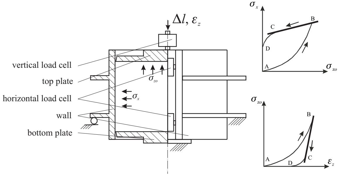
**Fig. 2.** Uniaxial compression apparatus and determination of modulus of elasticity.
