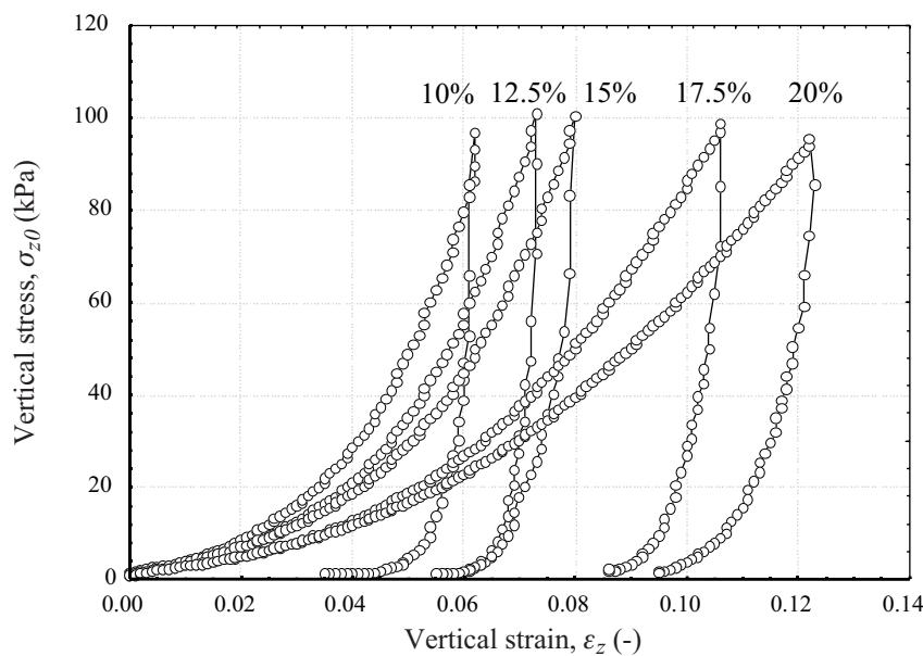
**Fig. 3.** Stress - strain relationships for uniaxial compression of wheat of five levels of moisture content.
