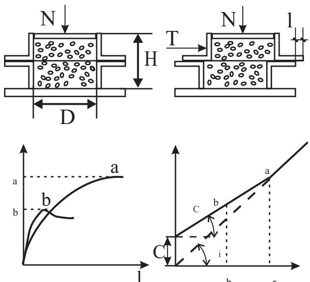
**Fig. 1.** Direct shear apparatus and determination of strength parameters based on the preconsolidation stress,  $\sigma_r$ .
