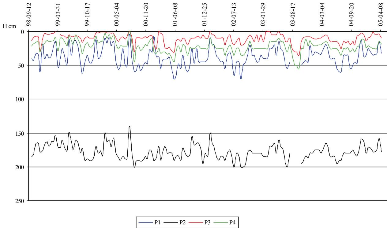
Fig. 1. The level of groundwater table in piezometers in the area of the nature preserve 'Międzyrzeki' between 1998 and 2005.
