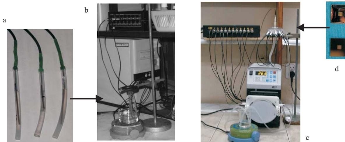
**Fig. 1.** Potassium sensors applied in work: a – medium-size ISEs, b – measuring set-up applying medium-size ISE, c – potassium-selective BSC sensor (on the left) and BSC silicon chip without polymeric membrane (on the right) and d – flow-through system applying BSC sensors.
