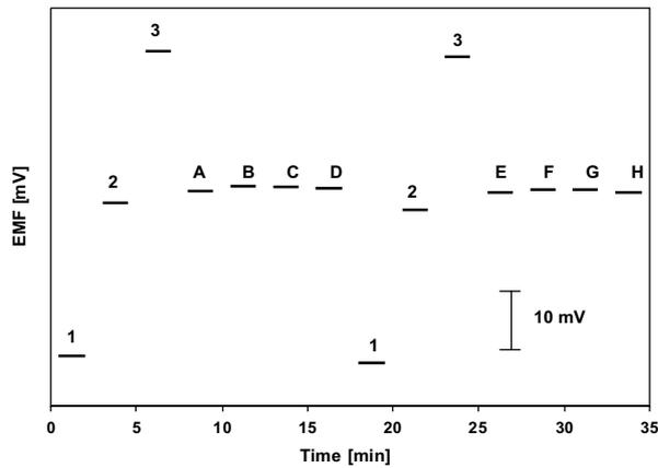
Fig. 3. Response behaviour of medium-size  $K^+$ -ISE in soil extracts (A-H) and calibrating solutions (1, 2, 3).
