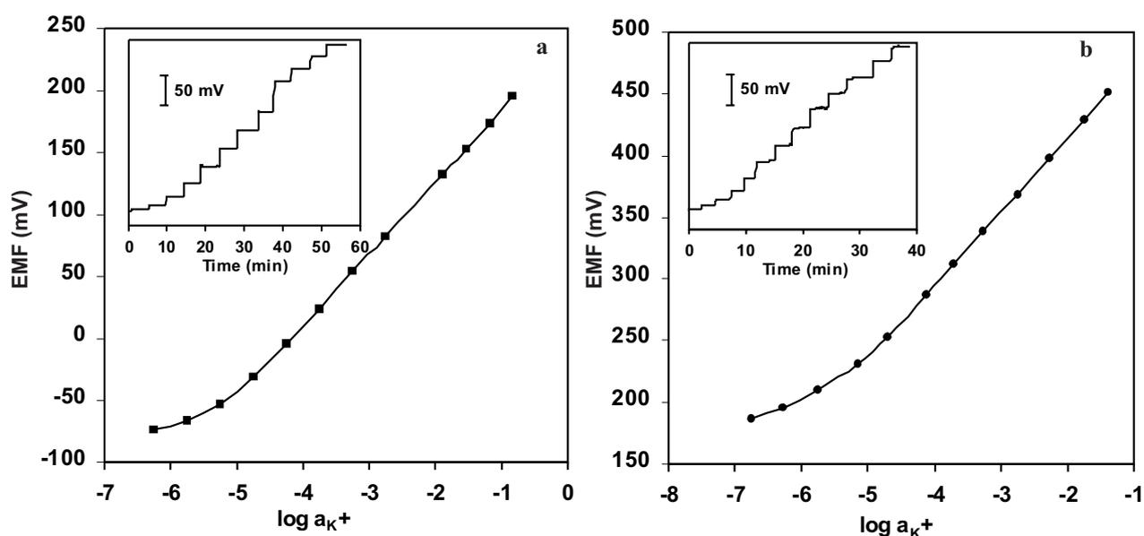
**Fig. 2.** Potentiometric response to changes in potassium concentration observed in 0.5 M BaCl<sub>2</sub> solutions for: a – medium-size  $K^+$ -ISE and b – miniaturized  $K^+$ -BSC sensors.
