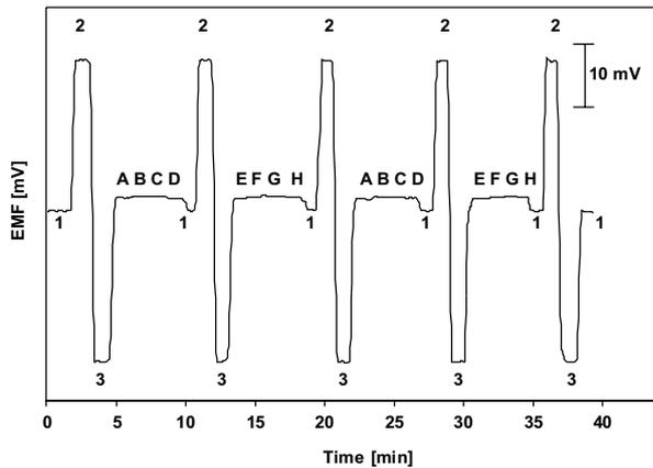
Fig. 4. Response behaviour of miniaturized  $K^+$ -BSC sensors in soil extracts (A-H) and calibrating solutions (1, 2, 3).
