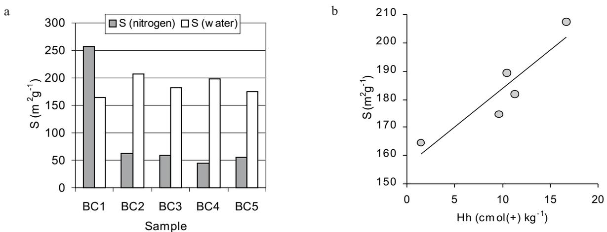
**Fig. 3.** Specific surface areas (SSA) of brown coals obtained from water vapours ( $S_w$ ) and nitrogen ( $S_{N_2}$ ) adsorption data using the BET method (a), relations between the specific surface area ( $S_w$ ) determined using the water vapours adsorption isotherm and the hydrolytic acidity (Hh) (b).
