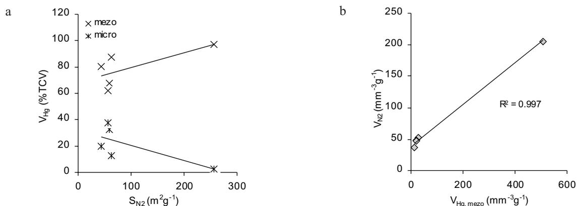
**Fig. 5.** Nitrogen surface area ( $S_{N_2}$ ) vs. the mezo- ( $V_{mezo}$ ) and micropore ( $V_{micro}$ ) volume of investigated coals (a); the regression between nitrogen pore volume ( $V_{N_2}$ ) and mezopore volume ( $V_{mezo}$ ) obtained from mercury porosimetry data (b).
