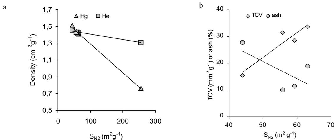
**Fig. 4.** Relation between the nitrogen specific surface area ( $S_{N_2}$ ) and density (a) (triangle - specific density ( $\rho_s$ ) measured by helium pycnometer, square - bulk density ( $\rho_b$ ) measured using MIP), and the total cumulative volume (TCV) (rhombus) and the ash content (circle) of brown coals (b).
