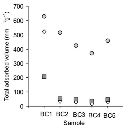
**Fig. 6.** Comparison of the pore volume (TPV) of coal samples determined from mercury porosimetry (diamonds), nitrogen (grey squares) and water vapour (grey circles) adsorption data.
