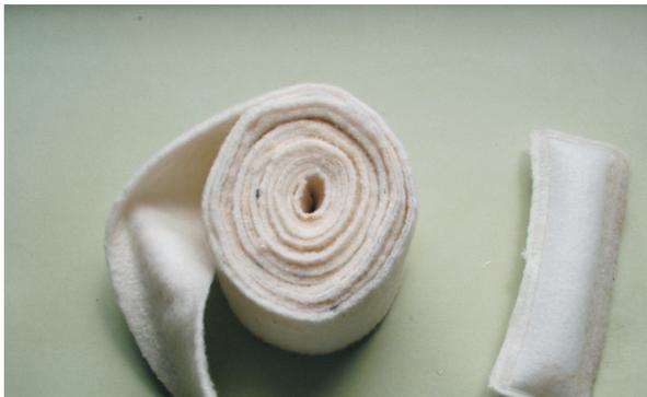
**Fig. 2.** Geocomposite made of non-woven geotextile with superabsorbent (SAP). On the right – small strip of the geocomposite swelled after water has been absorbed.
