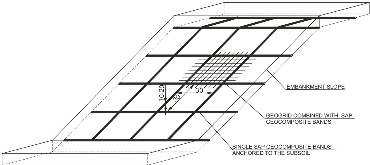
Fig. 7. Possible arrangements of geocomposite with SAP applied on slopes.
