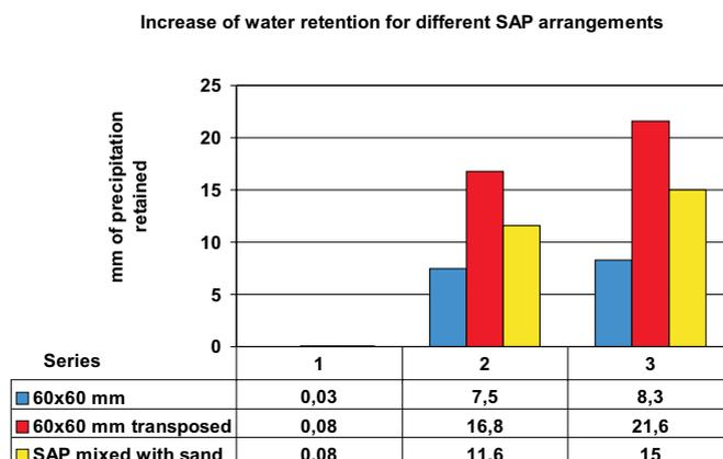
**Fig. 1.** Additional retention of water from precipitation in sand with SAP for different SAP arrangement in a column test. Theoretical sorption possibilities of SAP amount used in tests – 30 mm of rainfall.
