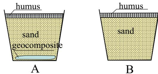
**Fig. 3.** Arrangement of humus, sand layers and SAP geocomposite position for preliminary application tests: A – container with a strip of geocomposite containing SAP; B – control container without superabsorbent; layers thickness: humus – 20 mm, sand – 300 mm, geocomposite – *ca.* 50 mm.
