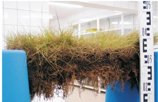
**Fig. 4.** Grass root system developed on a subsoil with (left) or without (right) SAP geocomposite.
