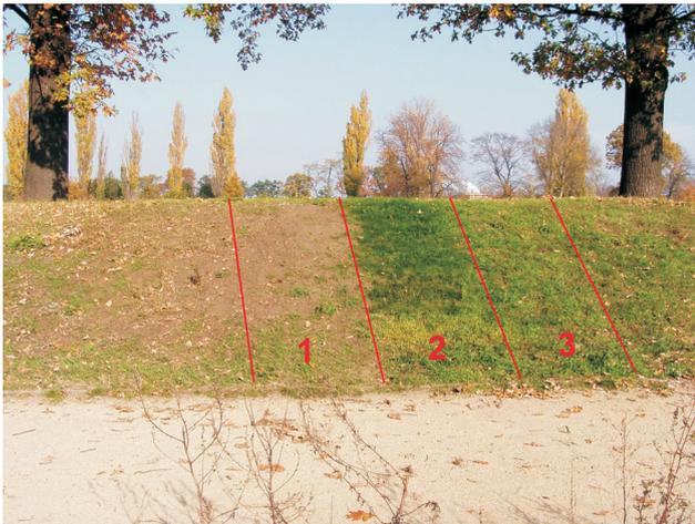
**Fig. 5.** Test application of geocomposite with SAP on a flood embankment slope.
