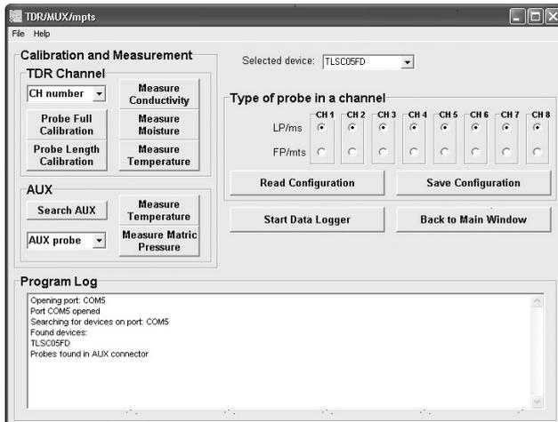
Fig. 2. Operation window for TDR/MUX/mpts meter.
