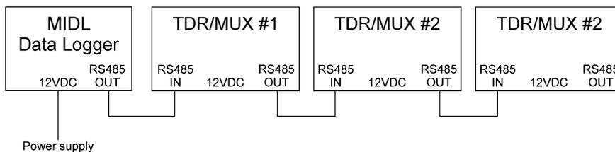
**Fig. 6.** Example connections of the measurement system consisting in a MIDL Data Logger and three TDR/MUX devices connected in series.
