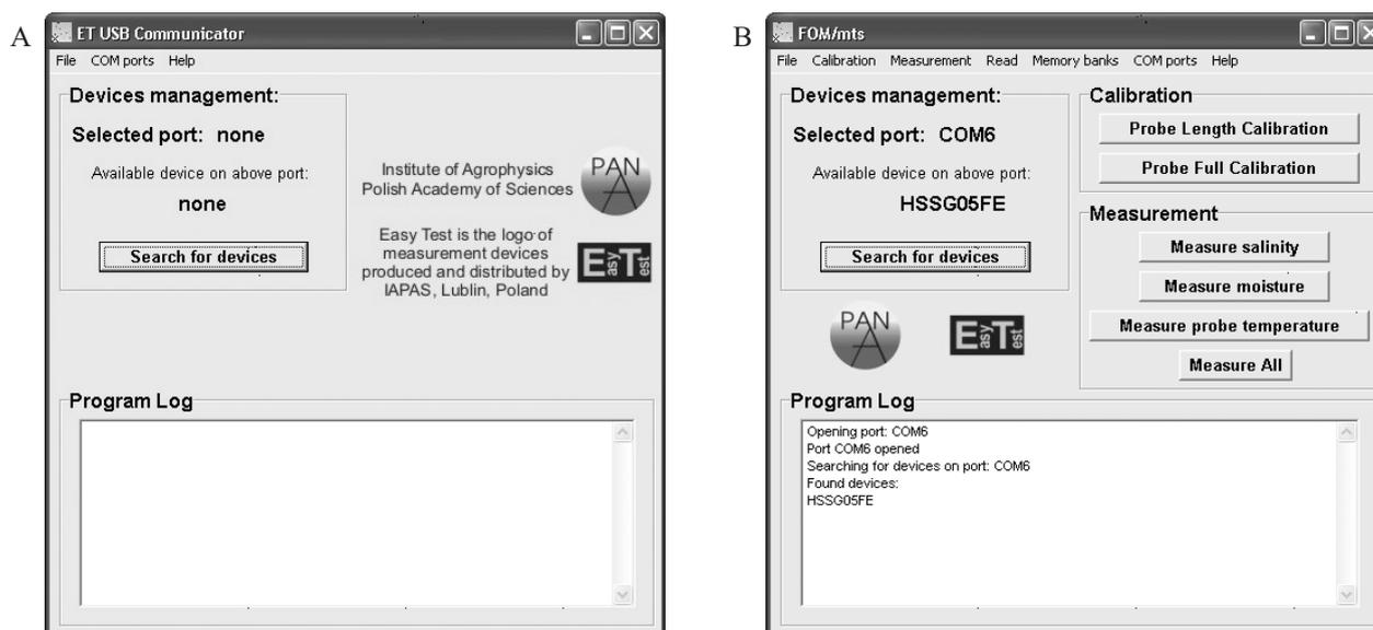
**Fig. 1.** The ET USB Communicator window: A – program entry window common for all devices, B – operation window for FOM/mts handheld meter.
