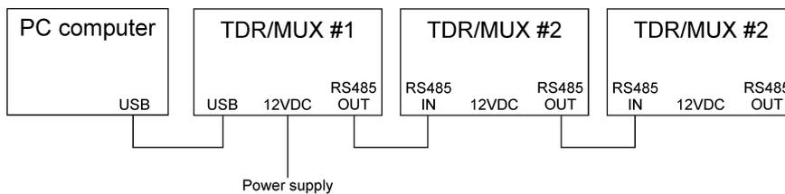
**Fig. 5.** Example connections of the measurement system consisting in a PC computer and three TDR/MUX devices connected in series.
