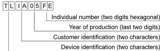
**Fig. 4.** Serial numbers of the measurement devices from the IA PAS, Lublin.
