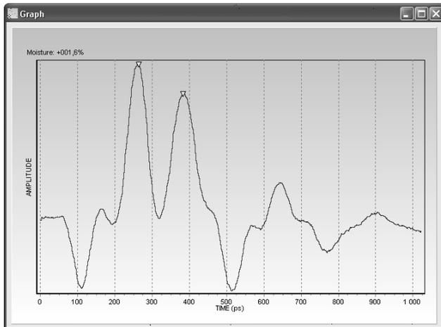
Fig. 3. TDR reflectogram from FP/mts probe connected to FOM/mts or TDR/MUX/mpts device controlled by 'ET USB Communicator'.
