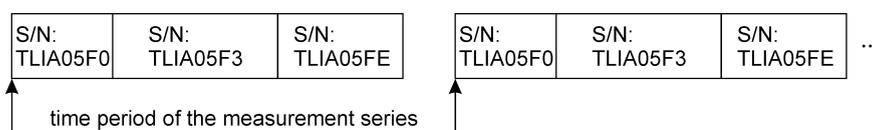
**Fig. 7.** Example of the sequence of measurements and time distance between the measurement series for three TDR/MUX/mts devices identified by various serial numbers.
