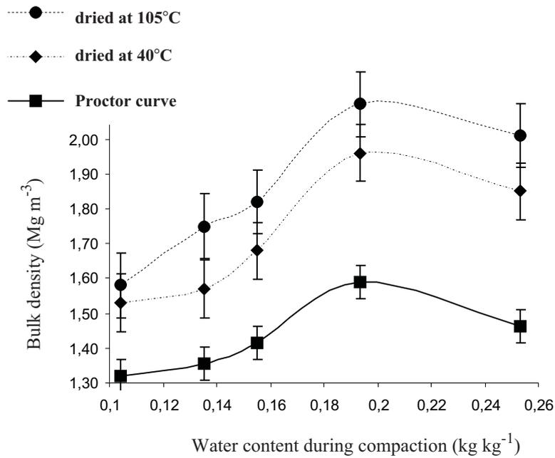
**Fig. 3.** The Proctor curve and the corresponding potential shrinkage curves (representing bulk densities) after drying at 40 and 105°C for the quaternary clay (Qc) versus water content during compaction test. Mean bulk density values with their standard deviations.
