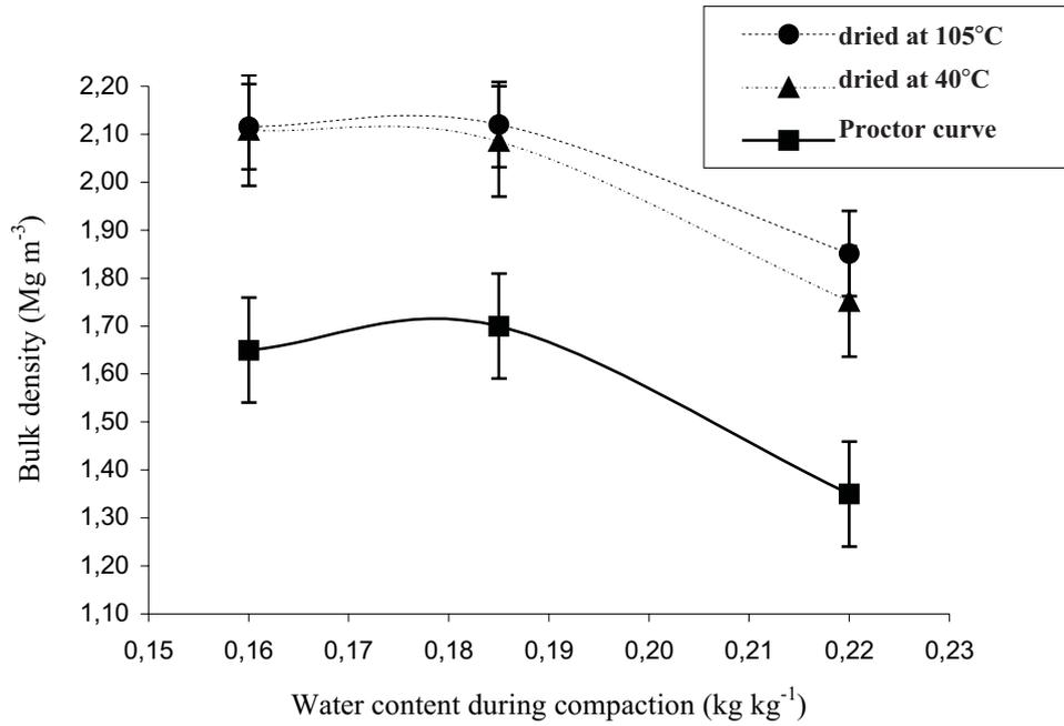
**Fig. 2.** The Proctor curve and the corresponding potential shrinkage curves (representing bulk densities) after drying at 40 and 105°C for the silty loam from Germany (Sl) versus water content during compaction test. Mean bulk density values with their standard deviations.
