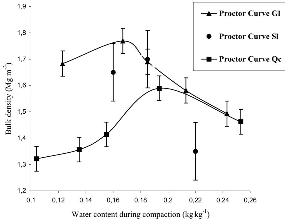
Fig. 1. The Proctor curves for the materials under study. Mean bulk density values with their standard deviations.
