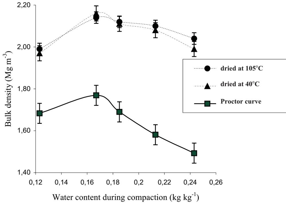
**Fig. 4.** The Proctor curve and the corresponding potential shrinkage curves (representing bulk densities) after drying at 40 and 105°C for the granite loam (GI) versus water content during compaction test. Mean bulk density values with their standard deviations.
