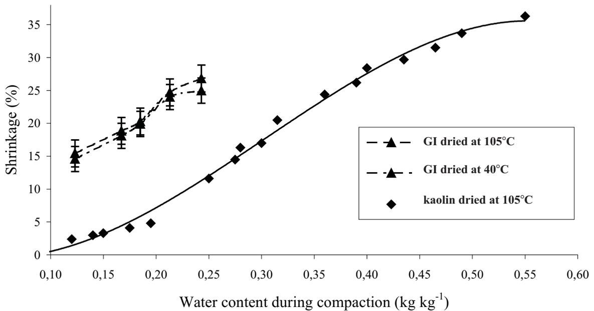
**Fig. 5.** Comparison of the kaolin potential shrinkage curve at 105°C expressed as percentage of volume change (calculated by us on the basis of the results of Bauer *et al.*, 2001) with analogous curves obtained by us for the granite loam at 40 and 105°C.
