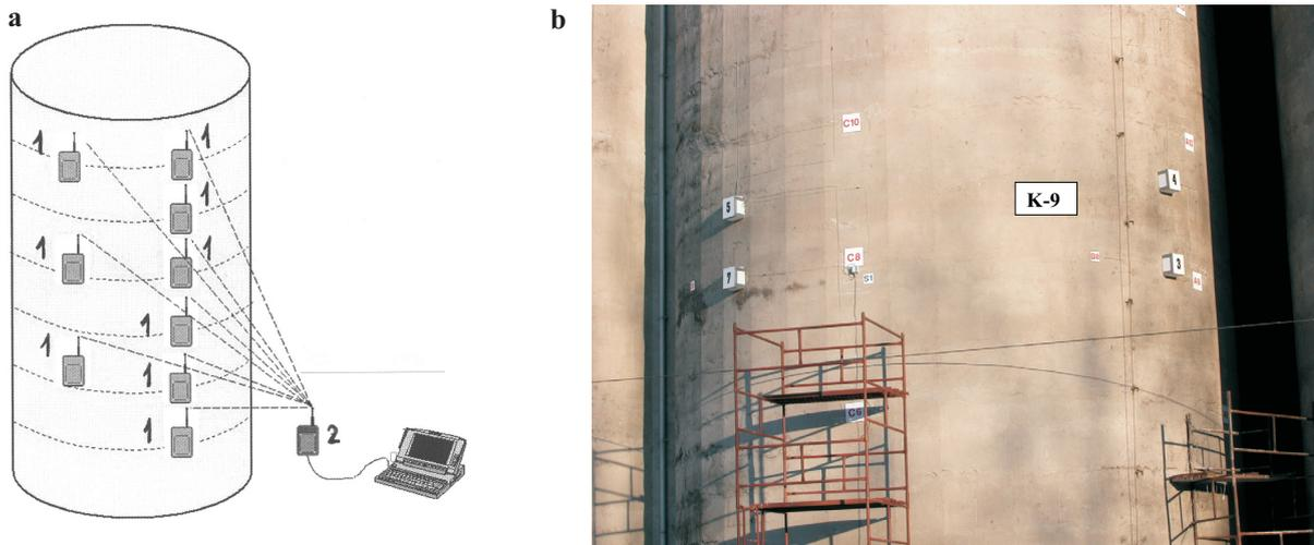
**Fig. 1.** Cylindrical silo bin structure during monitoring: a) scheme of wireless transmission: 1– transceivers, 2 – main station connected with computer; b) view of tested silo bin K–9 in Białystok Elevator.
