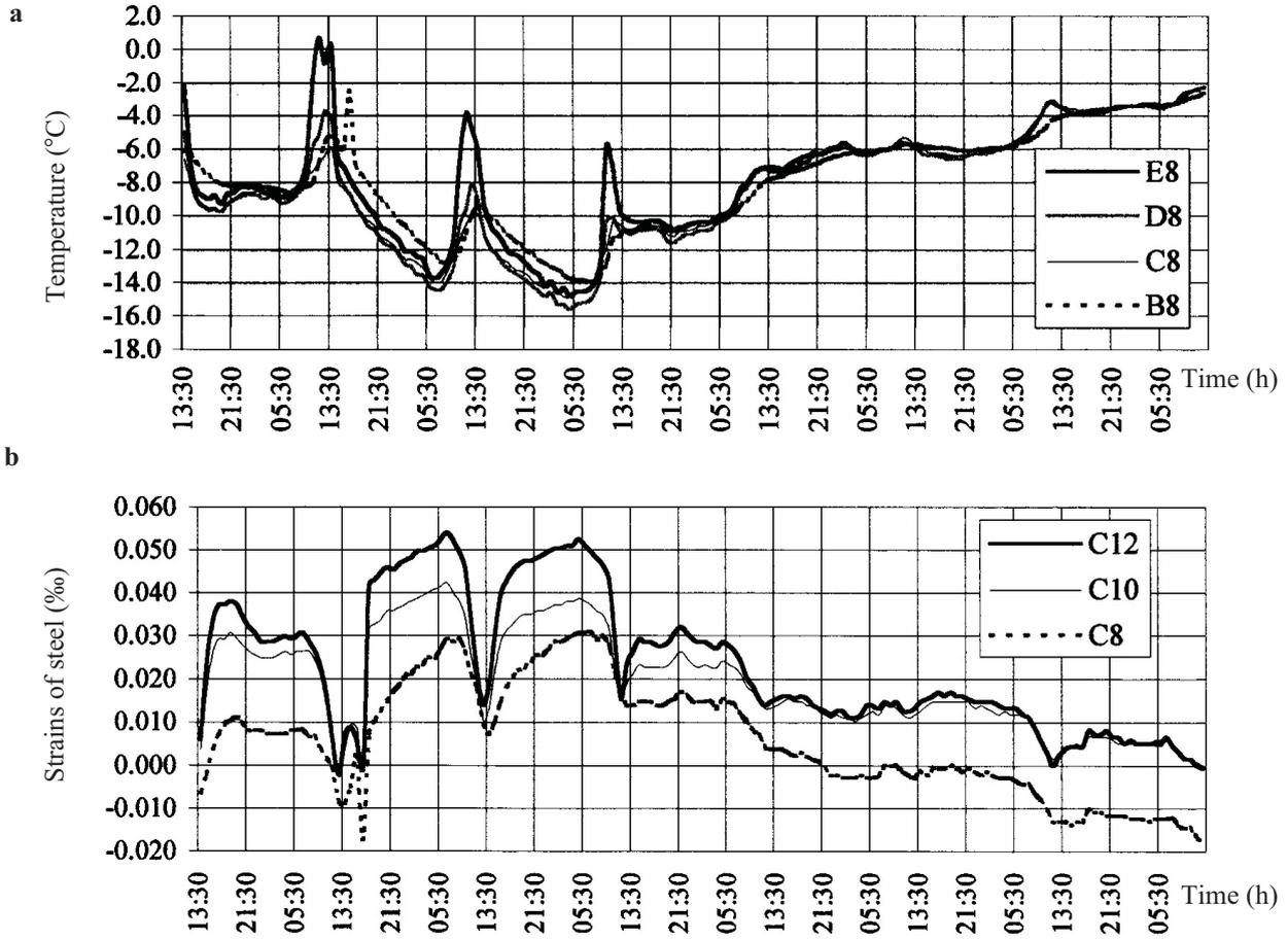
Fig. 3. Temperature distributions on silo battery perimeter (December 2002) (a) and corresponding thermal strain changes in reinforcing steel at selected test points (b) (Łapko, 2005).
