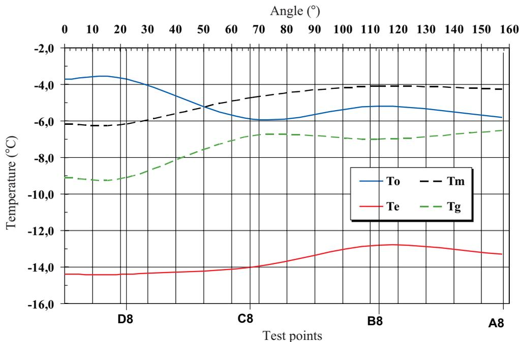
Fig. 6. Wall temperature distribution over the wall perimeter taken in computer simulations;  $T_o$ ,  $T_e$  – external surface temperature at the start and the end of monitoring, respectively,  $T_m$  – mean wall temperature;  $T_g$  – temperature difference at the wall thickness.
