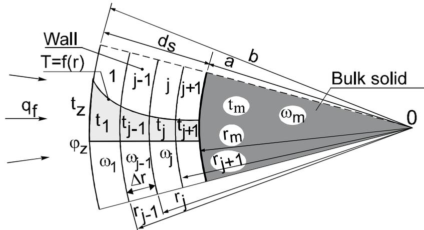
Fig. 4. Assumptions for the numerical computation of temperature in the system: silo wall – bulk solid (Łapko and Prusiel, 2001);  $T = f(r)$  temperature function against silo wall radius.
