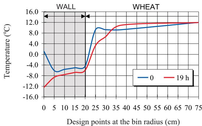
Fig. 5. Temperature distribution along the radius of silo bin.
