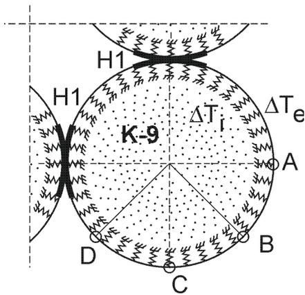
**Fig. 7.** Scheme for FEM analysis of silo battery using discrete model of interaction between wall structure and bulk solid.
