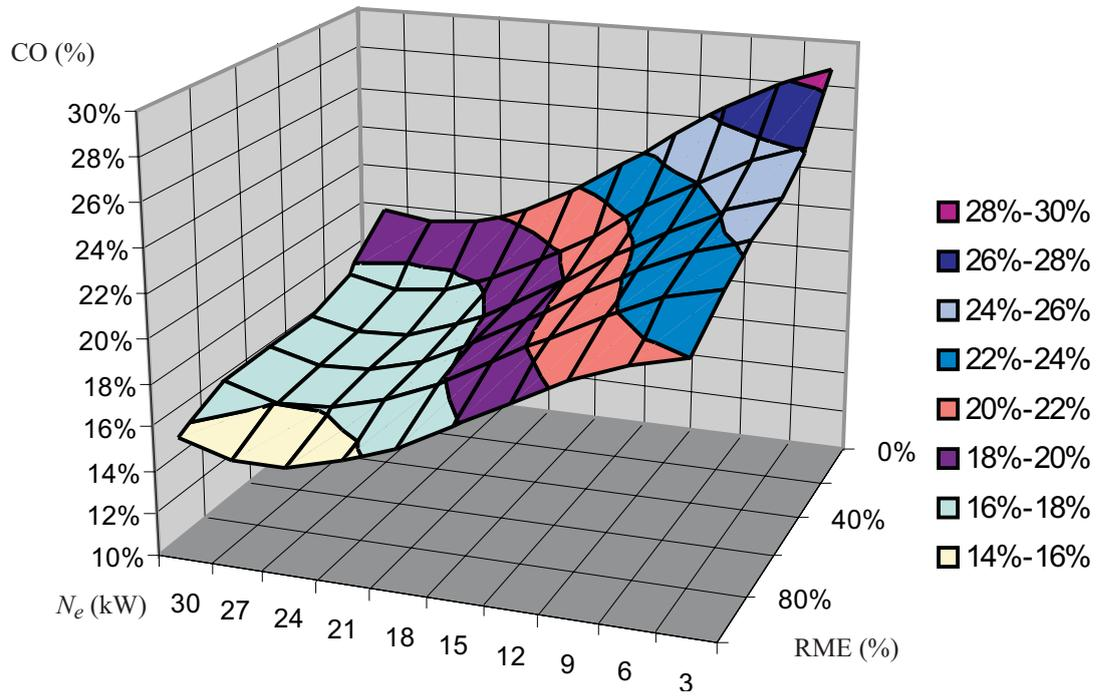
Fig. 4. Graph of CO ( $N_e$  RME) (%) regression 2000 r.p.m.
