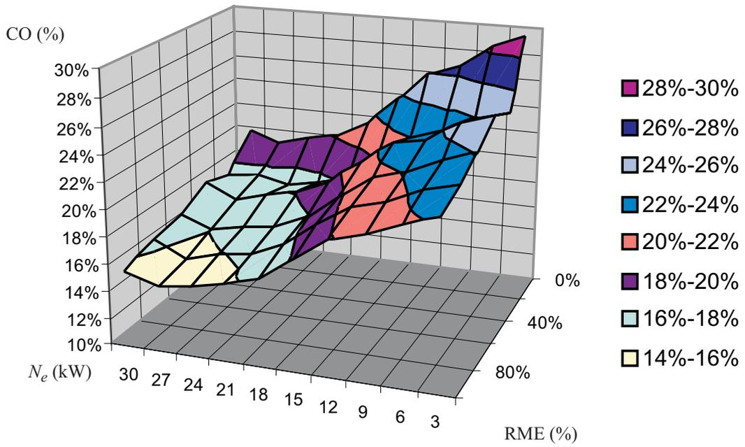
Fig. 2. Graph of CO (%) data for 2000 r.p.m.
