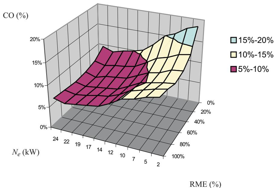
Fig. 1. Graph of CO (%) data for 1600 r.p.m.
