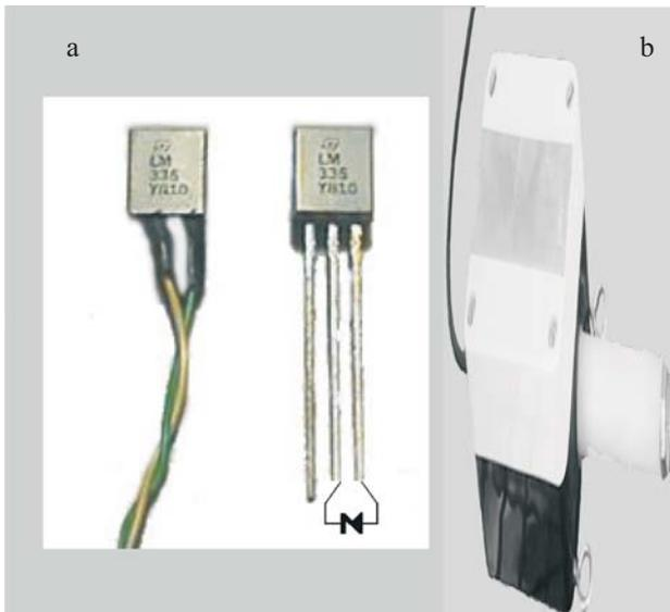
Fig. 3. Temperature sensor (a) and relative humidity sensor (b).
