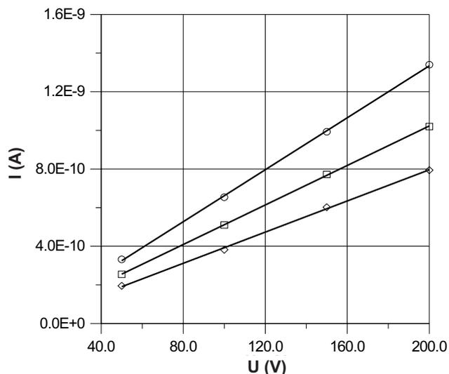
Fig. 1. The dependence of current passing through the sample on voltage, for sugar beet seeds of cultivars: Intera (filed seeds) (○), Polina (coated seeds) (□) and Remona (encrusted seeds) (◇), at average moisture content of 9.39%.
