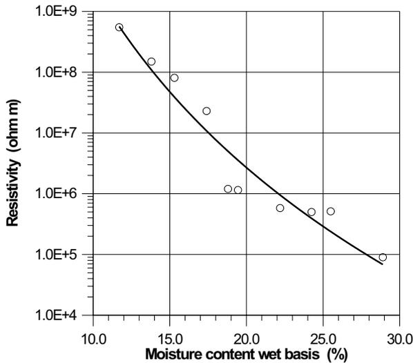
**Fig. 3.** The dependence of resistivity on moisture content wet basis for *Amaranthus hypochondriacus* at an average bulk density of  $760.4 \text{ kg m}^{-3}$ .
