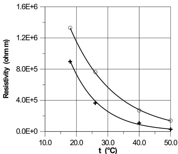
Fig. 2. The resistivity temperature dependencies for corn grains hybrids of Fabullis (○) at the moisture content wet basis of 16.9% and of Raissa (+) at 17.34%.
