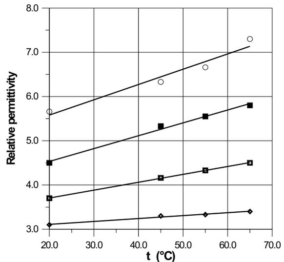
**Fig. 4.** The temperature dependencies of relative permittivity for wheat grains of Jubilejná variety at 2 MHz for moisture contents wet basis of: 12.5 (◇), 15.2 (□), 22.1 (■) and 26.3% (○).
