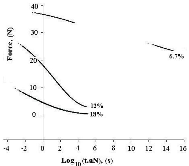
**Fig. 6.** Master curve obtained for chickpea kernels at 6.7, 12, and 18% moisture content.
