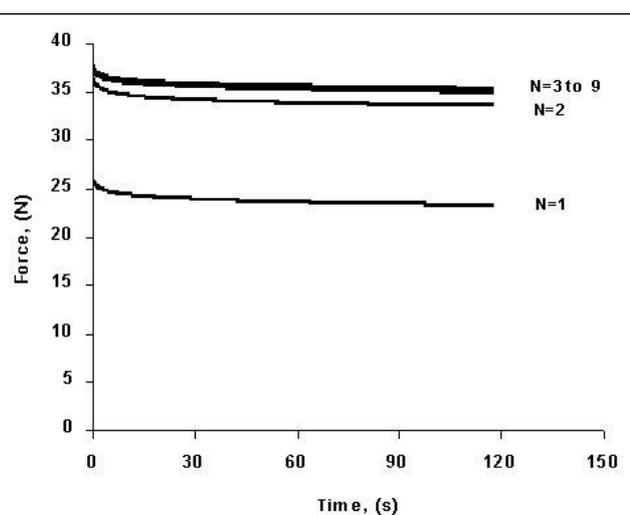
**Fig. 2.** Relaxation force behaviour of the same chickpea kernel subjected to nine successive relaxation tests at moisture content of 6.7%.
