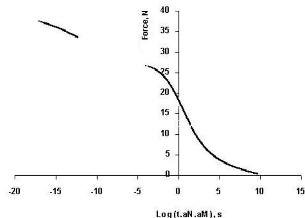
**Fig. 7.** Master curve obtained for estimating the relaxation force of chickpea kernels at moisture contents between 6.7 and 18% and number of loadings from 1 to 9 cycles.
