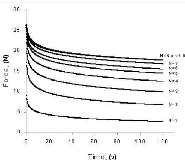
**Fig. 3.** Relaxation force behaviour of the same chickpea kernel subjected to nine successive relaxation tests at a moisture content of 12%.
