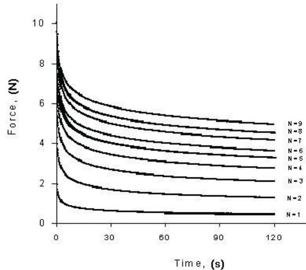
**Fig. 4.** Relaxation behaviour of the same chickpea kernel subjected to nine successive relaxation tests at a moisture content of 18%.
