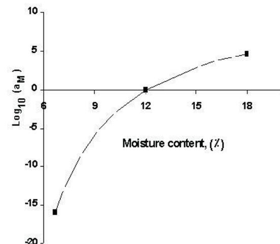
**Fig. 8.** Relationship between moisture content shift factor ( $a_M$ ) and moisture content of the chickpea kernels.
