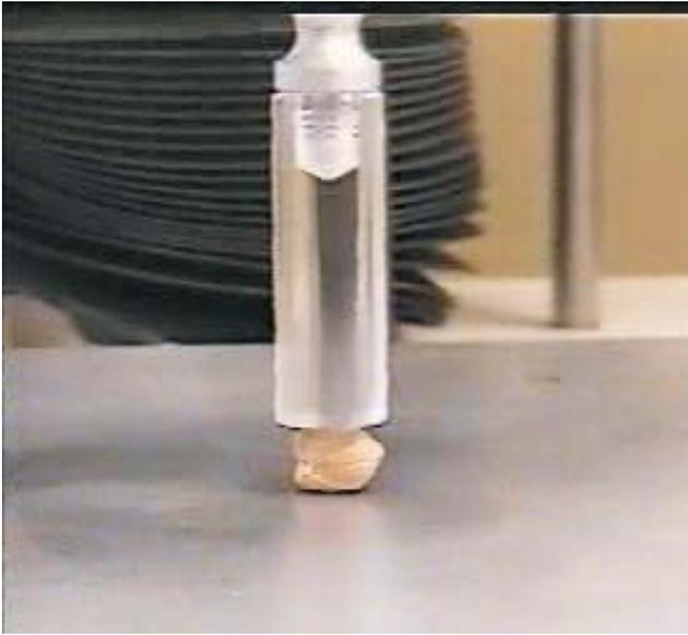
**Fig. 1.** Chickpea kernel loaded from the side between two parallel plates.
