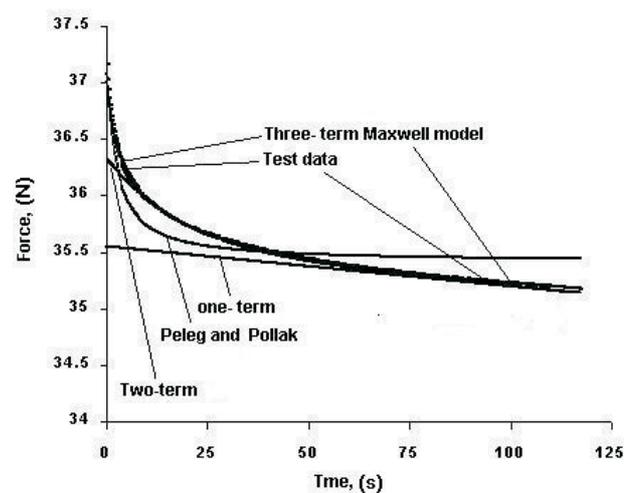
**Fig. 5.** Force relaxation behaviour of chickpea kernels at 6.7% moisture content as predicted by both the Maxwell and Peleg and Pollak models.
