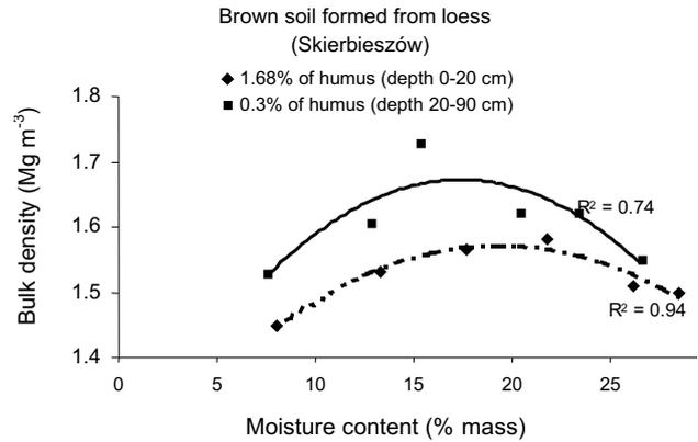
Fig. 2. Relation between bulk density and moisture content at different  $C_{org.}$  content in brown soil formed from loess.
