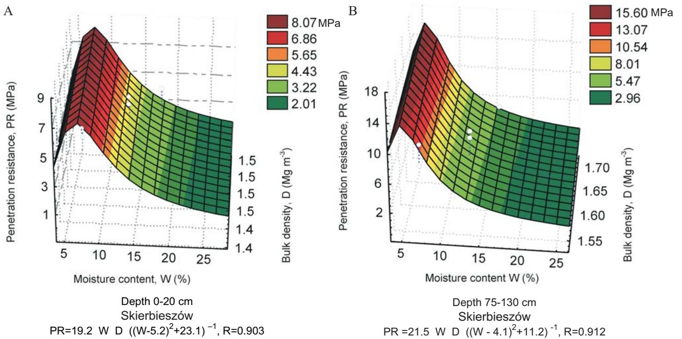
**Fig. 4.** Relation between penetration resistance (PR), moisture content (W), and bulk density (D), in grey-brown soil formed from loess: A) 2.1% and B) 0.2% of C<sub>org</sub> content. Legend presents penetration resistance values (MPa).
