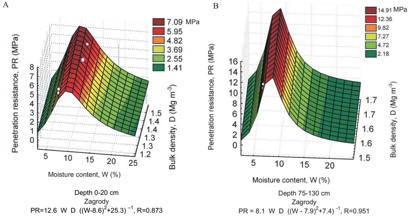
**Fig. 3.** Relation between penetration resistance (PR), moisture content (W), and bulk density (D), in grey-brown soil formed from loess: A) 2.1% and B) 0.2% of C<sub>org</sub> content. Legend presents penetration resistance values (MPa).
