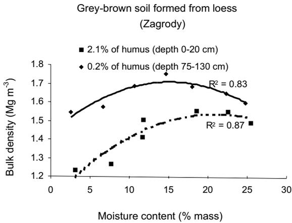
Fig. 1. Relation between bulk density and moisture content at different  $C_{org.}$  content in grey-brown soil formed from loess.
