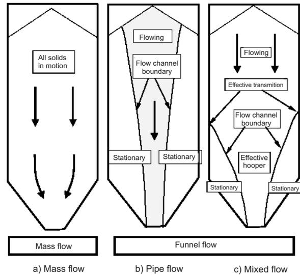
**Fig. 3.** Types of silo flow (Eurocode 1, part 4).
