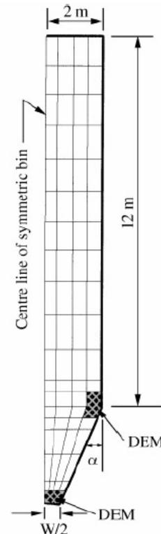
Fig. 6. Hybrid model between finite and discrete element methods (Jofriet *et al.*, 1997).
