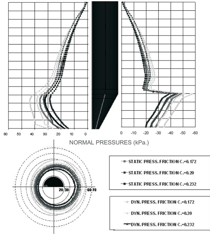
Fig. 10. Influence of the hopper eccentricity on static horizontal pressures.
