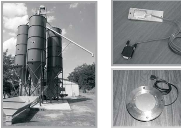
**Fig. 13.** Experimental silos in Madrid. The friction cell and the pressure cell.
