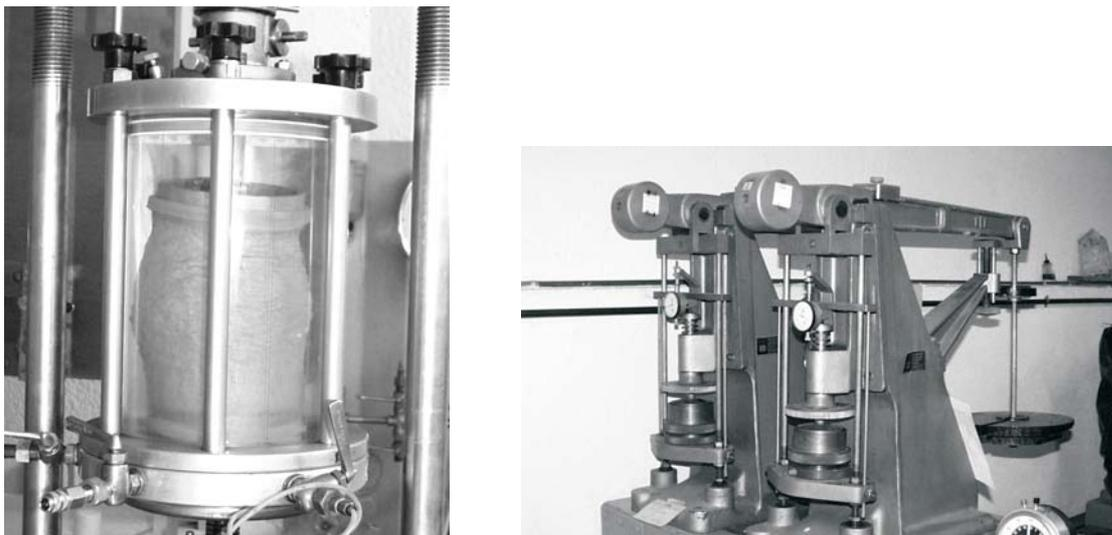
Fig. 11. Triaxial and oedometer tests.
