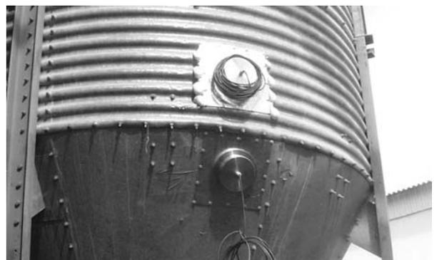
Fig. 12. Pressure cells in a silo with corrugated walls.
