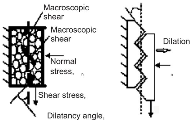
Fig. 5. The dilatancy phenomenon in silos horizontal overpressure during emptying (Zhang and Britton, 2003).
