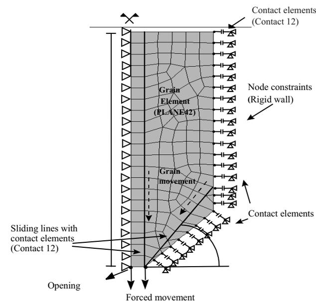
**Fig. 9.** A finite element model to simulate the silo emptying.
