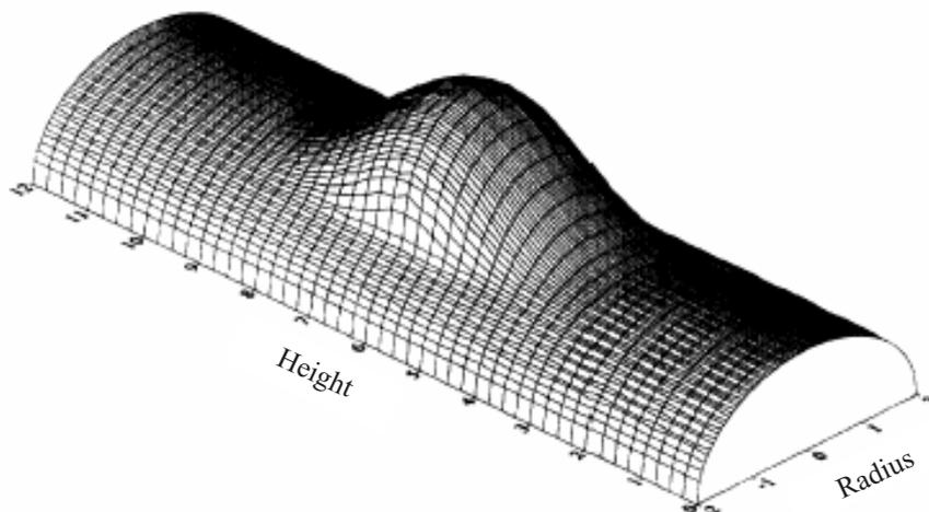
**Fig. 4.** Finite element simulation of a silo wall (Chen, Rotter and Ooi, 1998).
