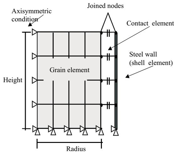
**Fig. 8.** A simple finite element model to simulate the grain and the wall at the same time.
