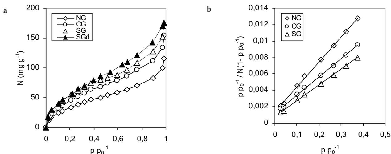
**Fig. 1.** Examples of water vapour adsorption data: original adsorption isotherms (a) and the BET plot for investigated soil samples (b). Abbreviation: NG, CG, SG – North, Central and South Gezira, N – amount of adsorbed water,  $p p_0^{-1}$  – relative pressure, white symbols – adsorption, black symbols – desorption.
