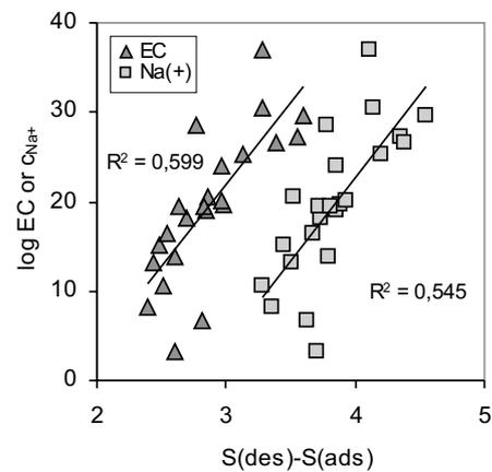
**Fig. 5.** Electrical conductivity (EC) or concentration of Na<sup>+</sup> versus the difference between values of the specific surface area (S) of investigated soil samples estimated from adsorption and desorption data of water vapour.
