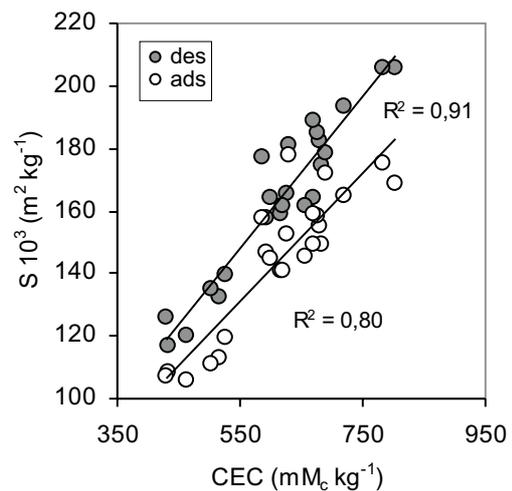
**Fig. 7.** The correlation between the specific surface area ( $S$ ) and the cation exchange capacity (CEC) for investigated soil samples. Abbreviation: see Fig. 1.
