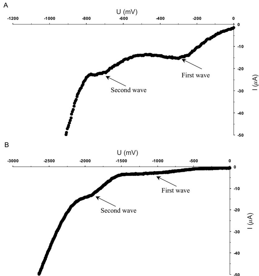
**Rys. 4.** Examples of current-voltage curves where two waves can be observed. These waves can be evidence that the reduction of molecular oxygen is not the unique electrochemical reaction in the system. A) three-electrode system in soil 565; soil water content 53.7%; B) three-electrode system in soil 606; soil water content 40.2%.
