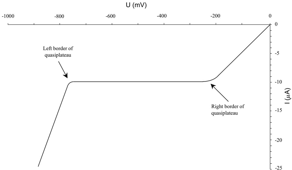
Fig. 2. Idealized current-voltage curve and definition of right and left borders of quasiplateau.
