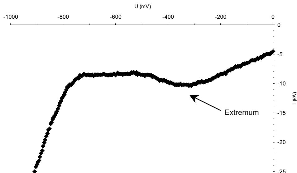
**Fig. 3.** Example of a current-voltage curve (soil No. 568; soil water content 46.7%) obtained with the three-electrode system. There is a relative extremum in the range of potentials of quasiplateau.
