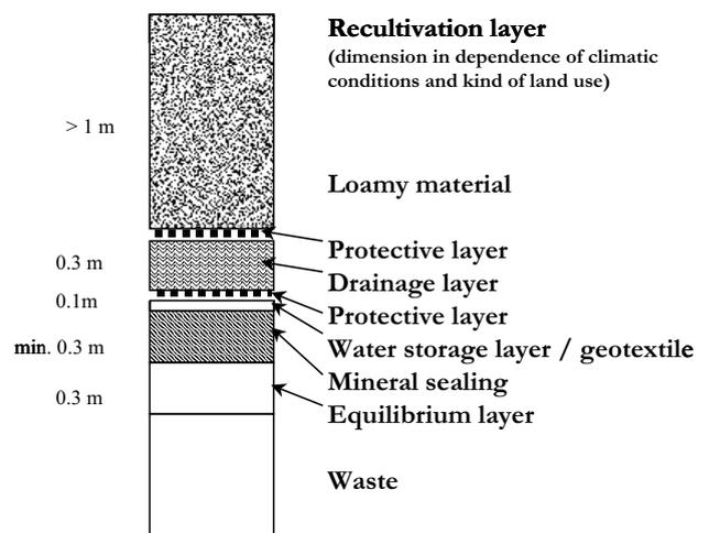
**Fig. 5.** A schematic of the pore barrier as an unpermeable layer in the landfill capping.
