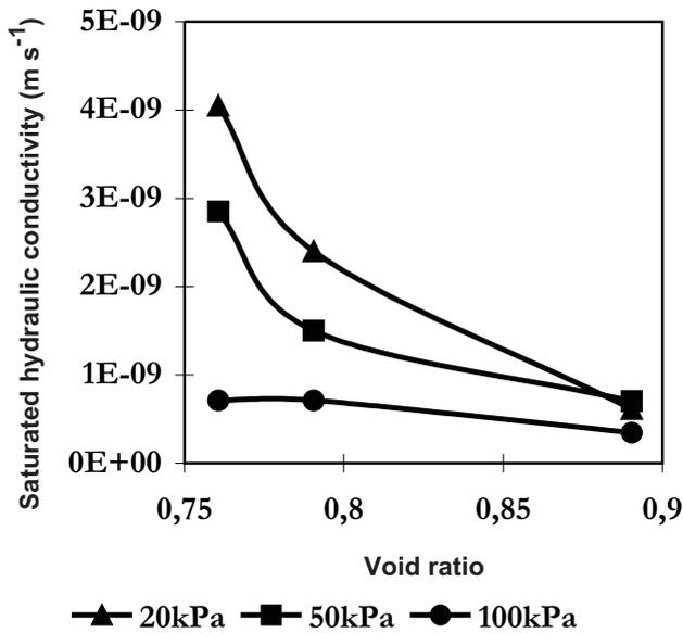
Fig. 3. Saturated hydraulic conductivity as a function of mechanical stress applied and the number of wetting and drying cycles for the same glacial till.
