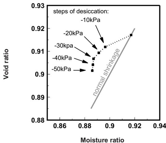
**Fig. 2.** Shrinkage behaviour of a glacial till soil at a given mechanical pre-stress of 30 kPa and consecutive drying.
