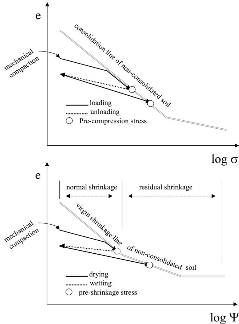
**Fig. 4.** Shrinkage and stress strain behaviour of soil samples (conceptual model according to Toll (1995)). Explanations: e - void ratio,  $\sigma$  - mechanical stress,  $\Psi$  - matric water potential.
