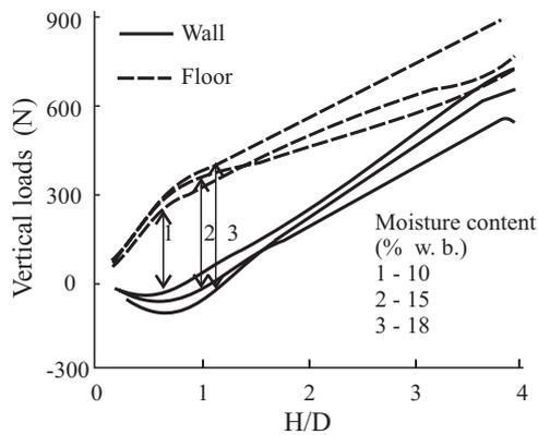
**Fig. 3.** Vertical wall and floor loads as affected by the height-to-diameter ratio ( $H/D$ ) during discharge for wheat at three moisture contents.
