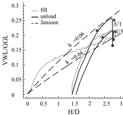
**Fig. 5.** Comparisons of experimental and predicted (Janssen) relations of vertical wall load-to-gross grain load ratio (VWL/GGL) to the height-to-diameter ratio (H/D) during fill and unload (U1 – first, U5 – fifth) cycles.
