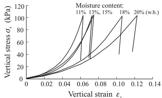
**Fig. 2.** Stress-strain relationships for uniaxial compression tests of wheat grain.
