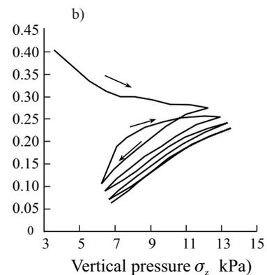
**Fig. 4.** The pressure ratio (a) and the coefficient of wall friction (b) versus the vertical pressure for wheat in succeeding loading-unloading cycles.
