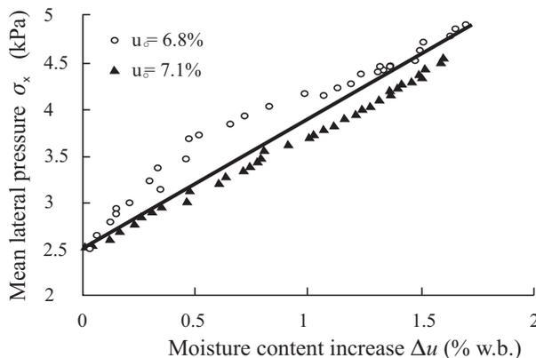
**Fig. 1.** Mean lateral pressure on the silo wall as influenced by moisture content increase.
