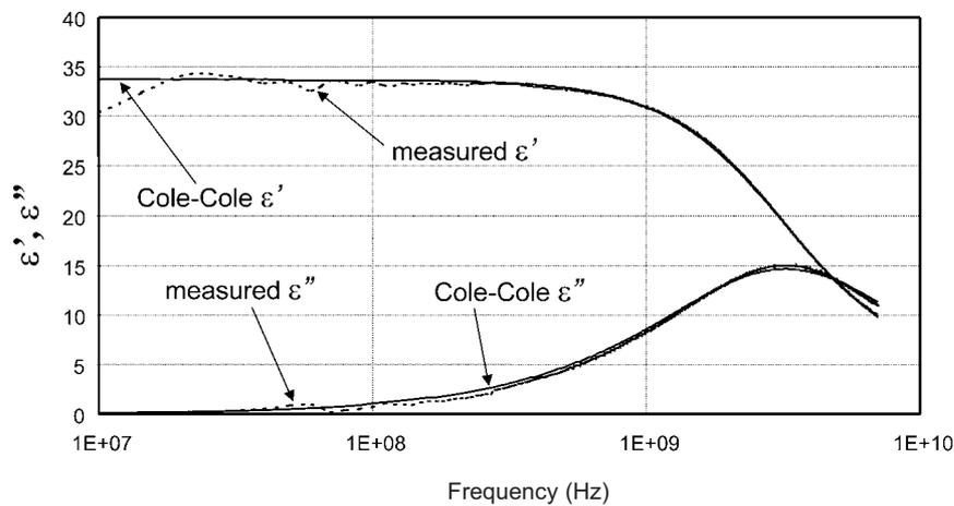
**Fig. 6.** Frequency change of real and imaginary parts of the complex dielectric permittivity of methanol for Cole-Cole modelled data and measured using Open-Ended Coaxial probe.
