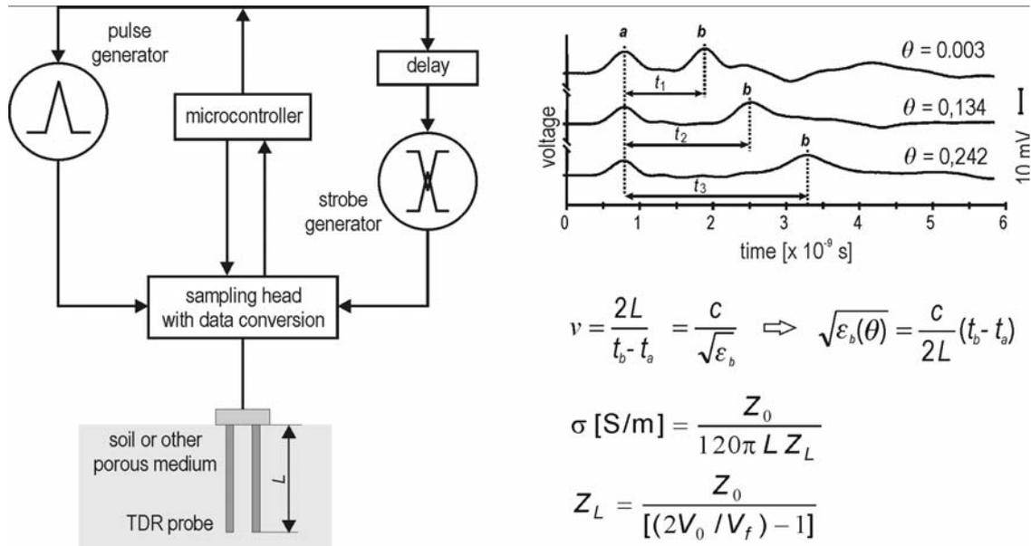
**Fig. 2.** Basic elements of the time domain reflectometer for determination of velocity of propagation of electromagnetic waves in porous media.
