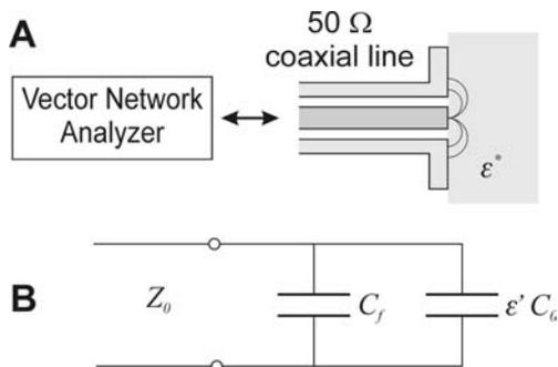
**Fig. 4.** A - Open-ended coaxial probe in the form of coaxial line open to the space with material of unknown dielectric permittivity  $\epsilon^*$ , B - modelling the discontinuity of electromagnetic field by lumped capacitances  $C_f$  and  $C_0$ .
