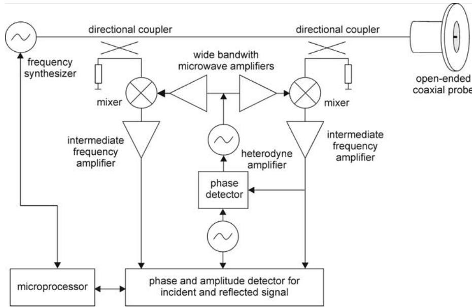
**Fig. 3.** Basic elements of the frequency domain reflectometer for determination of complex dielectric permittivity of porous media.
