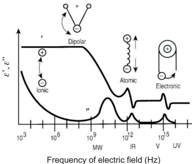
**Fig. 1.** Frequency response of dielectric mechanisms: MW, IR, V and UV are the microwave, infrared, visible and ultraviolet spectra respectively (HP AN 1217-1, 1992).
