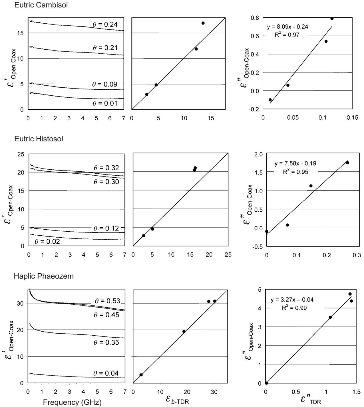
**Fig. 7.** Comparison of real,  $\epsilon'$ , and imaginary,  $\epsilon''$ , parts of the complex dielectric permittivity for the selected soils, calculated from the TDR and Open-Ended Coax probe measurements;  $\epsilon_{b\text{-TDR}}$  is the bulk dielectric constant measured by TDR.
