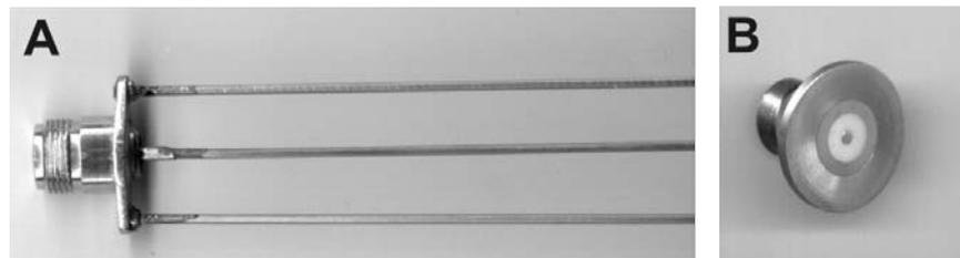
**Fig. 5.** A three-rod TDR probe (A), and an Open-Ended Coax probe (B) used in the measurement of dielectric permittivity of soils.
