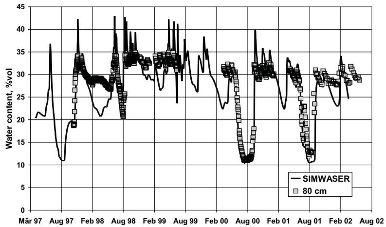
Fig. 5. Comparison of simulated and measured water content at 80 cm depth.
