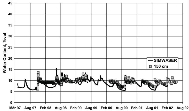
Fig. 6. Comparison of simulated and measured water content at 150 cm depth.
