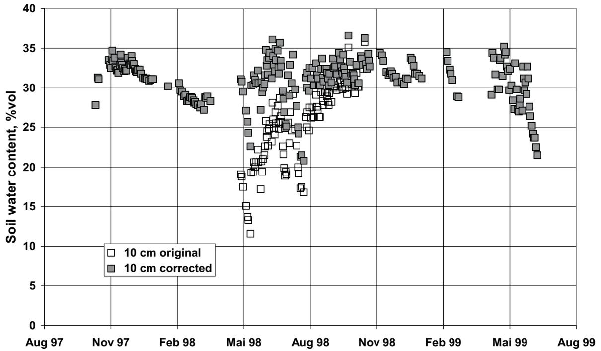
Fig. 1. Measured soil water content within the plough layer before and after correction.
