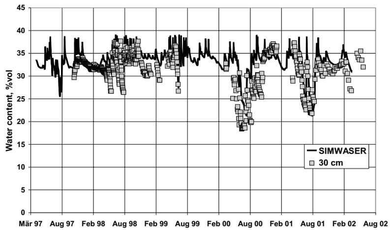
Fig. 4. Comparison of simulated and measured water content at 30 cm depth.
