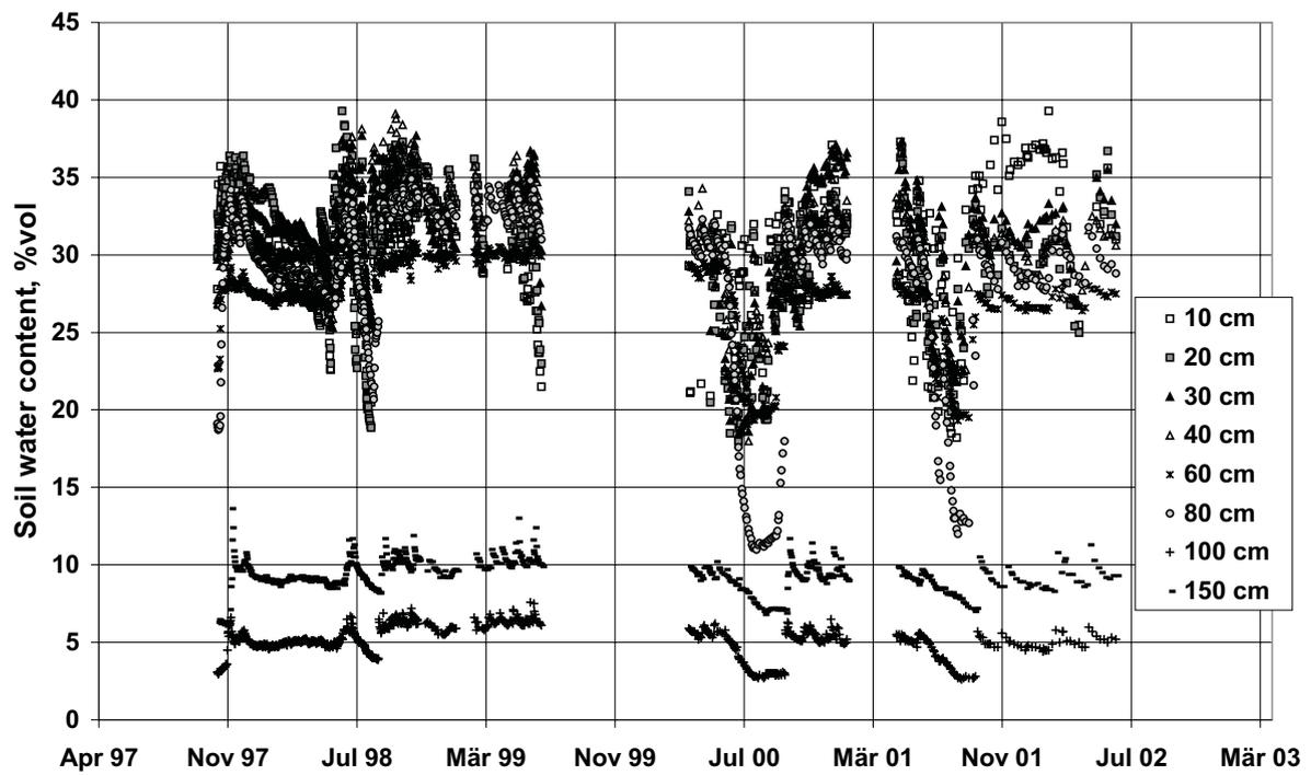
Fig. 2. Water content measurements with the EASY TEST FOM moisture meter.
