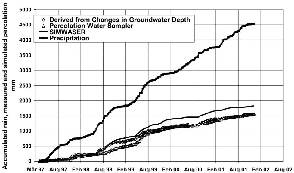
Fig. 8. Comparison of simulated and measured ground water recharge.
