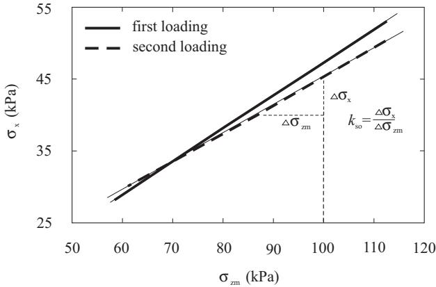
**Fig. 4.** Typical plot of the lateral pressure  $\sigma_x$  versus the mean vertical pressure  $\sigma_{zm}$  during first and second loading of the sample of seeds (rape seeds of moisture content of 6% w.b.).
