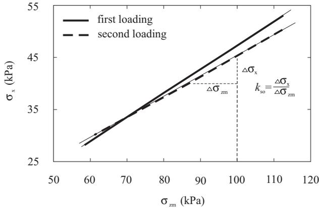
**Fig. 4.** Typical plot of the lateral pressure  $\sigma_x$  versus the mean vertical pressure  $\sigma_{zm}$  during first and second loading of the sample of seeds (rape seeds of moisture content of 6% w.b.).
