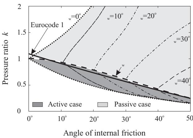
**Fig. 2.** Pressure ratio as the function of the angle of internal friction and the angle of wall friction for yielding at the wall (Horabik and Rusinek, 2000); — the pressure ratio according to Eurocode 1 (1996).
