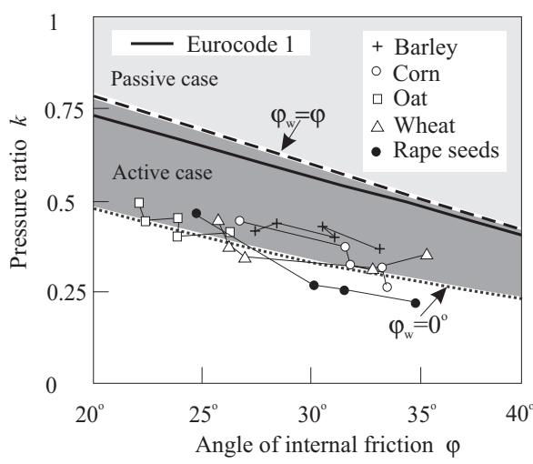
**Fig. 5.** Comparison of the experimental and theoretical values of the pressure ratio.
