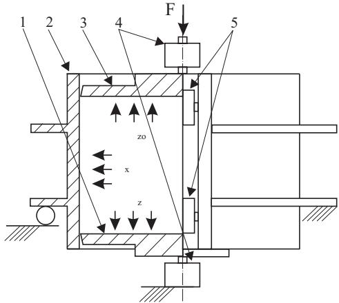
**Fig. 3.** Uniaxial compression tester: 1 – bottom plate, 2 – wall of the tester, 3 – top plate, 4 – load cells (vertical pressure), 5 – load cells (lateral pressure).
