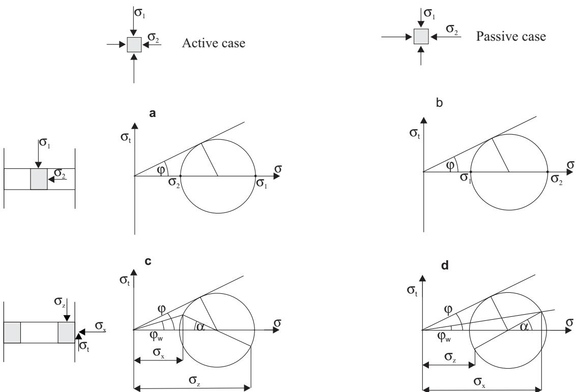
**Fig. 1.** Mohr's stress circles for: active case, yielding at the centre (a); passive case, yielding at the centre (b); active case, yielding at the wall (c); passive case, yielding at the wall (d).
