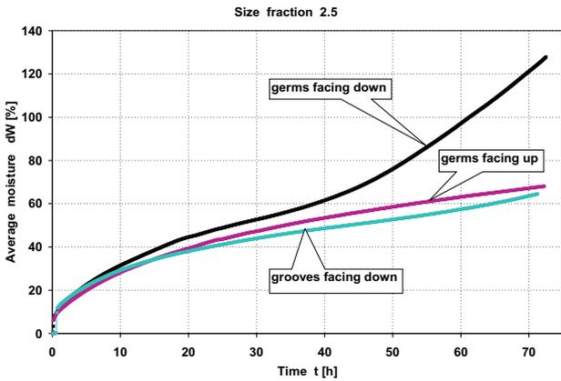
Fig. 7. Water intake rate in the wheat grain size fraction 2.5 for three kinds of placement on wet tissue.
