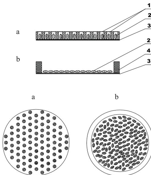
**Fig. 1.** Forms for grains: in the shape of a plate with holes for grains with their germs facing downwards and upwards (a), ring-like form for grains with their grooves facing downwards (b): 1 – wheat grains, 2 – metal ring, 3 – tissue, 4 – holes with diameters adequate for a particular grain fraction.
