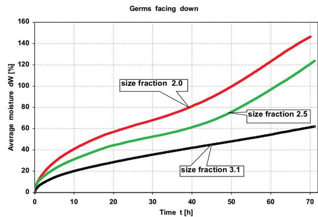
**Fig. 3.** Water intake rate in wheat grain of three size fractions, grain germs face down.
