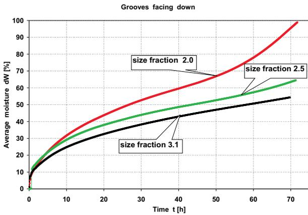
Fig. 5. Water intake rate in wheat grain of three size fractions, the grooves of the grains facing down.
