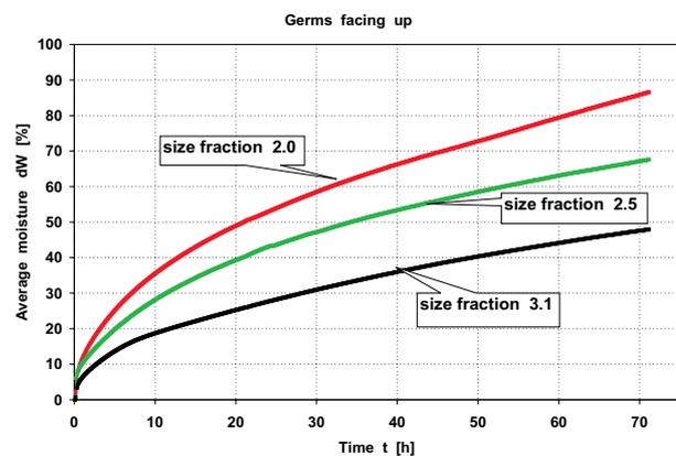
**Fig. 4.** Water intake rate in wheat grain of three size fractions, the germs of the grains facing up.
