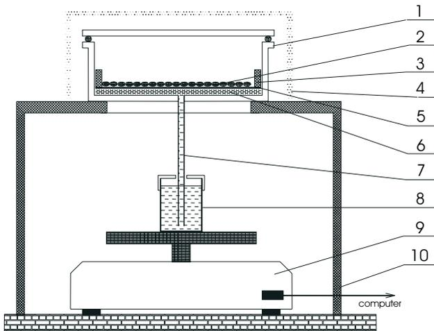
**Fig. 2.** Draft of the measurement unit: 1 – thermostatic container for grains, 2 – grains, 3 – ring, 4 – thermostatics (cover), 5 – tissue fixed to the ring, 6 – wet tissue, 7 – capillary, 8 – water container, 9 – electronic scales, 10 – support base for the container.
