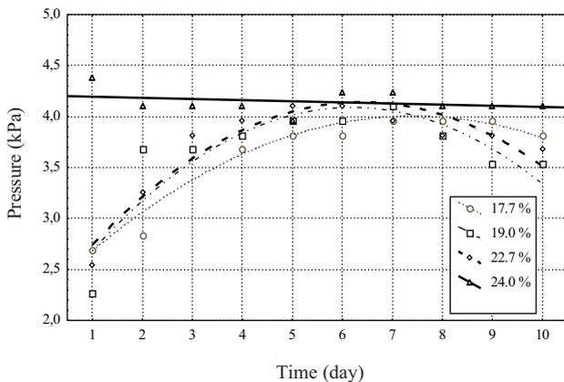
**Fig. 7.** Pressure against silo bottom as a function of storage duration.
