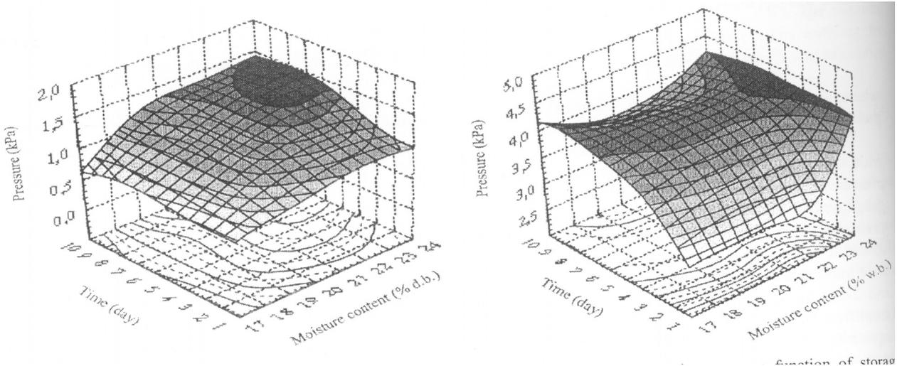
Fig. 5. Average pressure on the silo walls as a function of storage duration and grain moisture content. Fig. 6. Pressure against silo bottom as a function of storage duration and grain moisture content.
