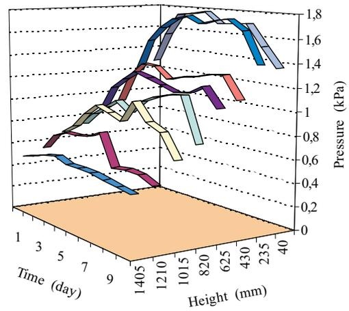
**Fig. 2.** Pressure exerted on the silo walls by barley grain with 13% d.b. moisture content.
