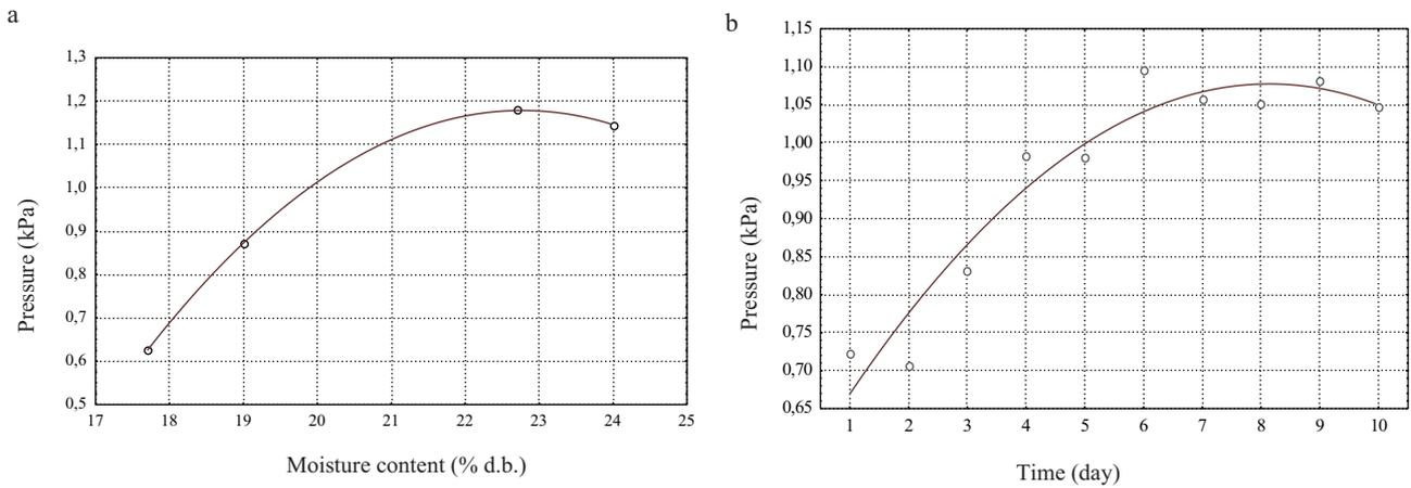
Fig. 4. Average values of pressure against silo walls versus: grain moisture content (a) and storage duration (b).
