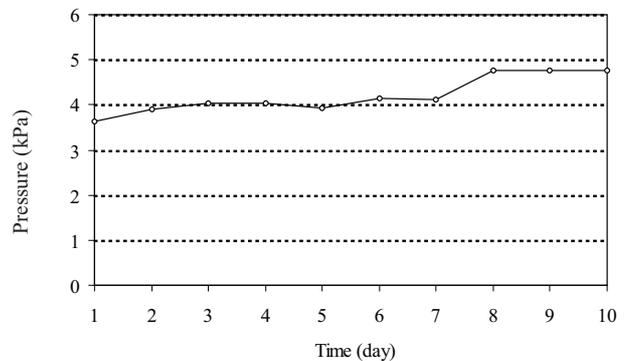
**Fig. 3.** Pressure exerted on the silo bottom by barley grain with 13% d.b. moisture content (measured in the silo axis).
