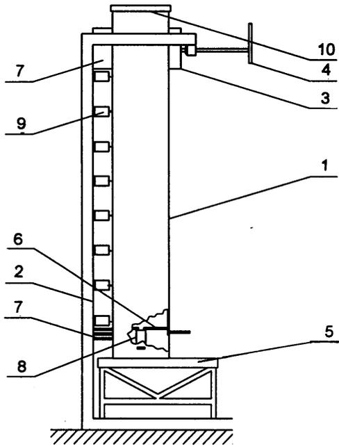
**Fig. 1.** Scheme of a measuring stand: 1 - cylindrical silo; 2 - frame; 3 - block; 4 - regulation mechanism; 5 - stand; 6 - bottom; 7 - spacing elements; 8, 9 - extensometrical sensors; 10 - cover.
