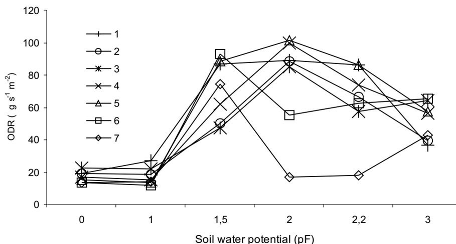
Fig. 2. Relationship between soil water potential (pF) and ODR.
