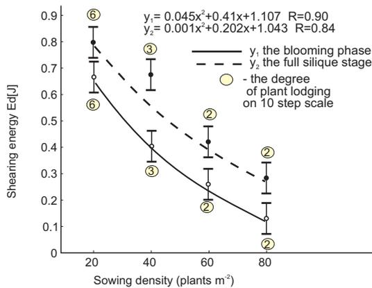
**Fig. 7.** Variation of shearing energy of Jupiter winter rape stalk with sowing density.
