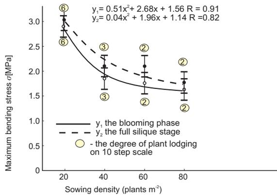
**Fig. 6.** Variation of maximum bending stress of Jupiter winter rape stalk with sowing density.
