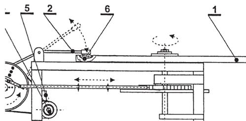
Fig. 3. Ram stand for multiple dynamic loads: 1 - rotating disc, 2 - beater ram, 3 - crank lever mechanism, 4 - motor, 5 - grain, 6 - spring latch mechanism.
