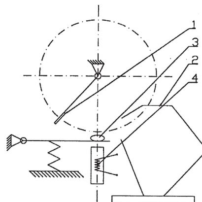
Fig. 2. Rotor stand for multiple dynamic loads: 1 - hitting plate, 2 - gauge, 3 - grain, 4 - electromagnet.
