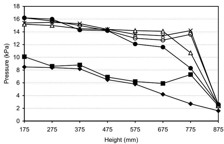
Fig. 3. Pressure values for triticale grain with moisture content: 13% w.b. (a), 16% w.b. (b), and 18% w.b. (c).
