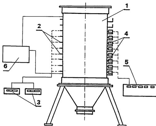
**Fig. 1.** Schematic diagram of the test station. 1 - silo, 2 - thermocouples, 3 - temperature gauges, 4 - strain gauges, 5 - silo wall load indicator with amplifier, 6 - thermostat.
