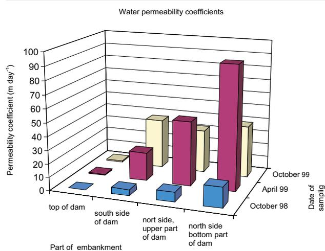
**Fig. 6.** Geometric averages of water permeability coefficients in a different parts of embankment and a different periods.
