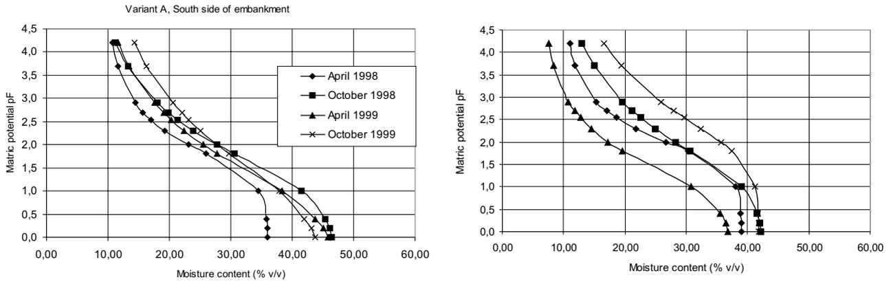
Fig. 2. Relationships between shapes of pF curves and the time period from the beginning of the experiment - variant A.
