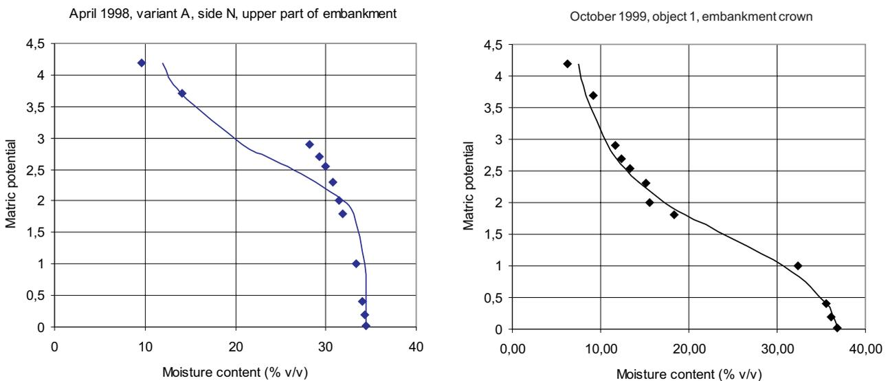
**Fig. 1.** Differences between the experimental points and curves smoothed with van Genuchten's formulae.
