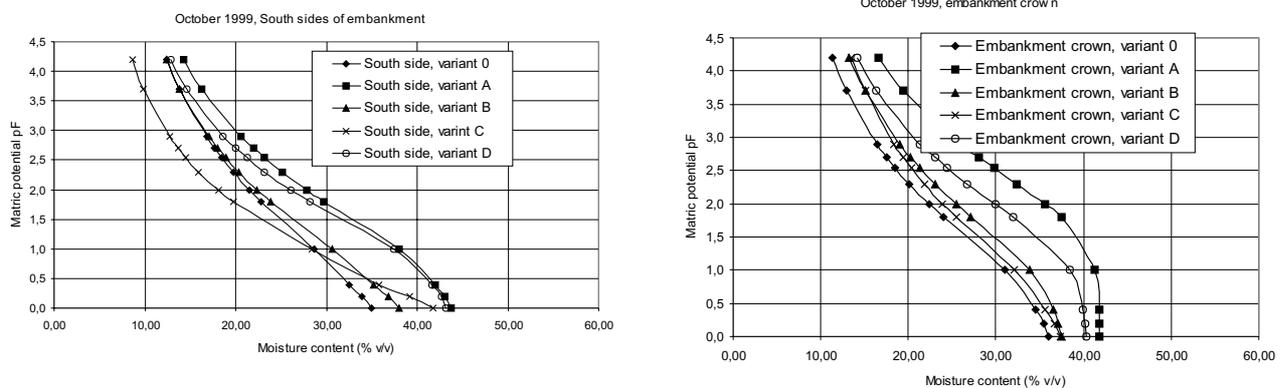
Fig. 5. The shape of pF curves of different variants describing the same parts of the embankment at the October 1999.
