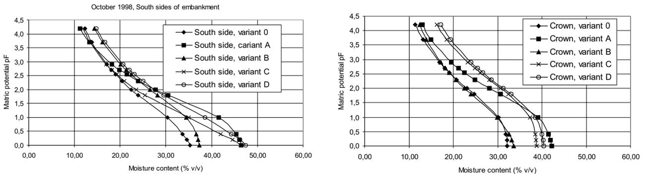
Fig. 4. The shape of pF curves of different variants describing the same parts of the embankment at the October 1998.
