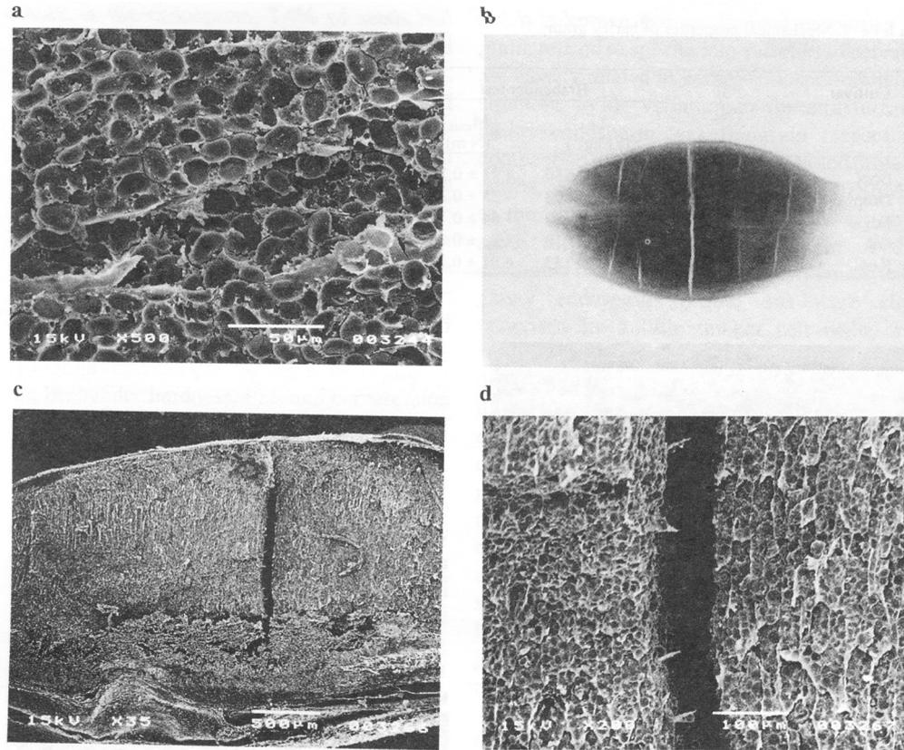
**Photo 2.** Micrographs of a meal kernel. SEM micrographs of a meal kernel (a), X-ray picture of a kernel (b), SEM micrographs of damage details: longitudinal section of a kernel (c), crack across endosperm (d).
