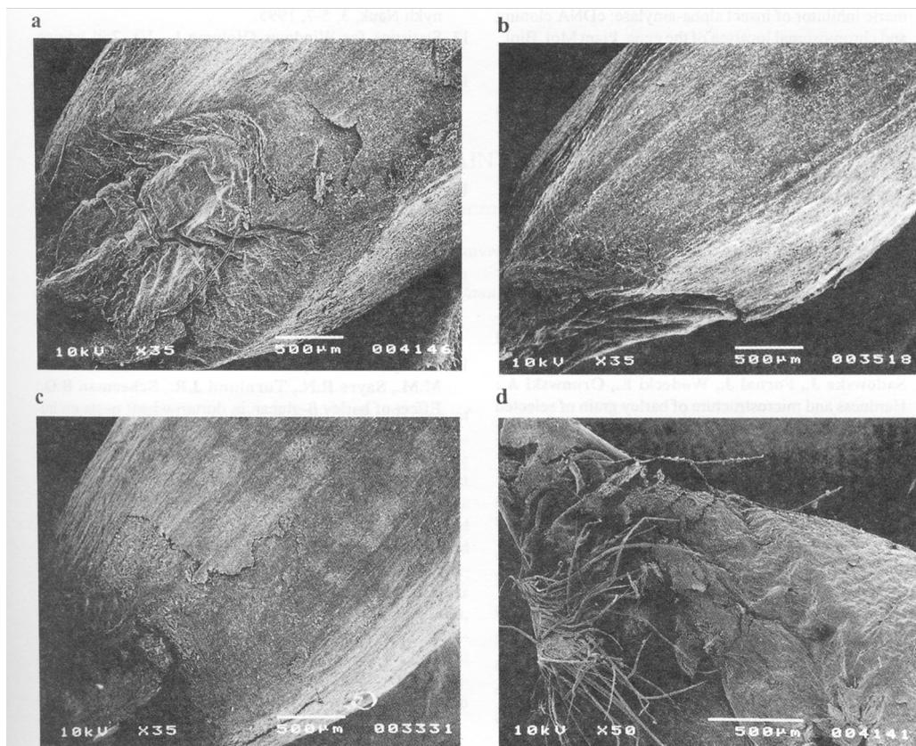
**Photo 3.** Micrographs of a meal kernel. SEM micrographs of a meal kernel (a), X-ray picture of a kernel (b), SEM micrographs of damage details: longitudinal section of a kernel (c), crack across endosperm (d).
