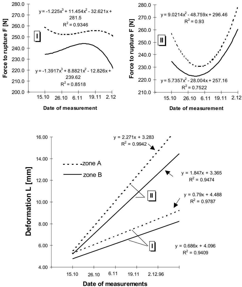
**Fig. 4.** Effect of storage time (date of measurements) and loading zone on force to rupture and deformation in I - natural conditions and II - room conditions.
