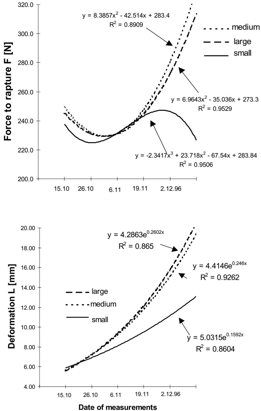
**Fig. 3.** Effect of storage time (date of measurements) and size of sugar beet roots on rupture force and deformation in room conditions.
