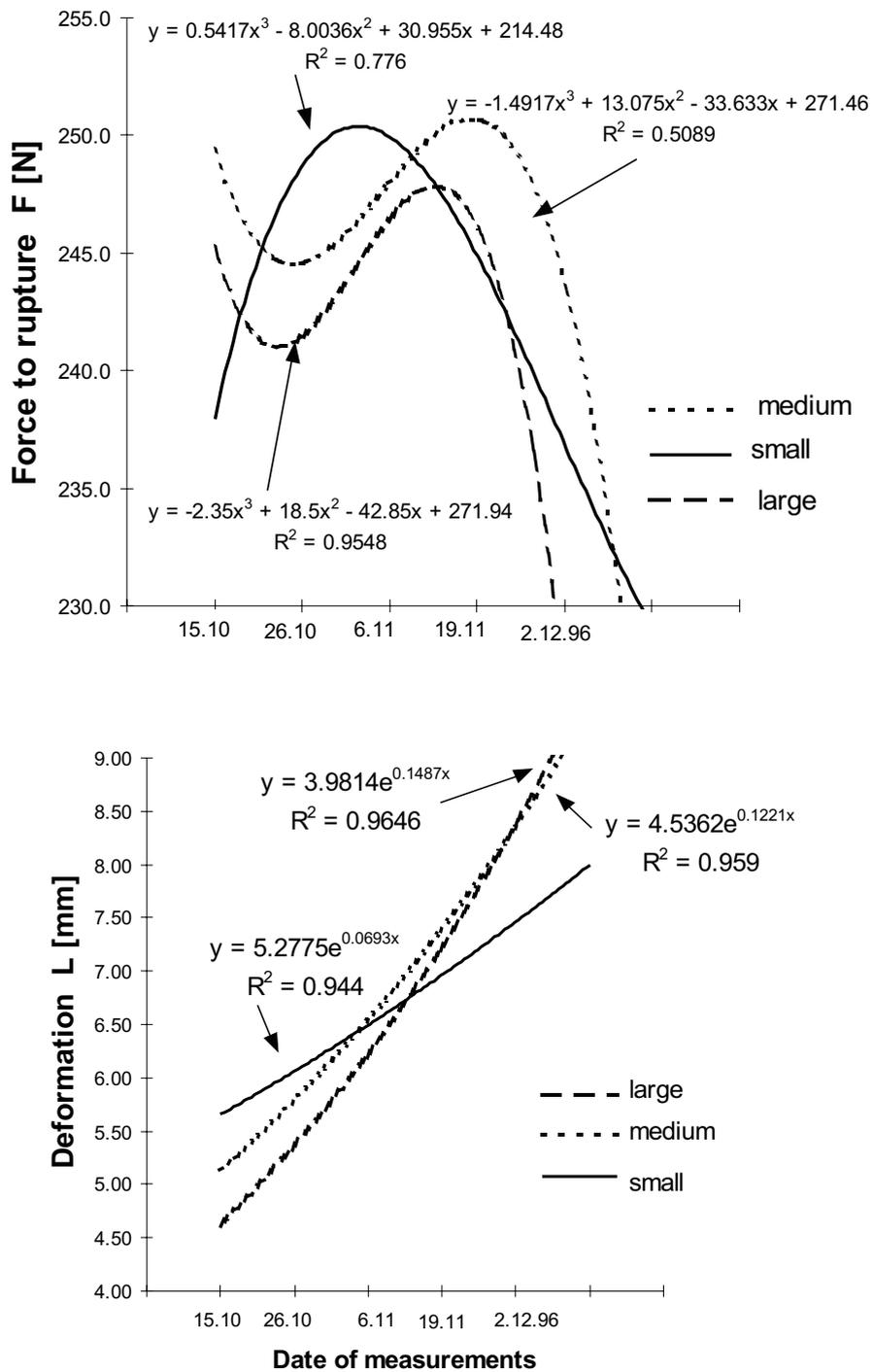
Fig. 2. Effect of storage time (date of measurements) and size of sugar beet roots on rupture force and deformation in natural conditions.
