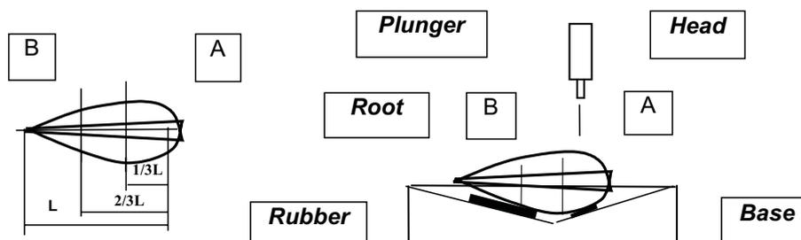
Fig. 1. Zones of sugar beet roots tested by 8 mm steel plunger: A -top zone , B - middle zone.
