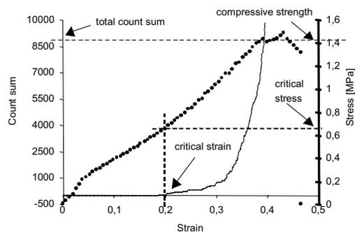
**Fig. 1.** The stress-strain curve (wide line) and the count sum - strain curve (narrow line) recorded in the experiment.
