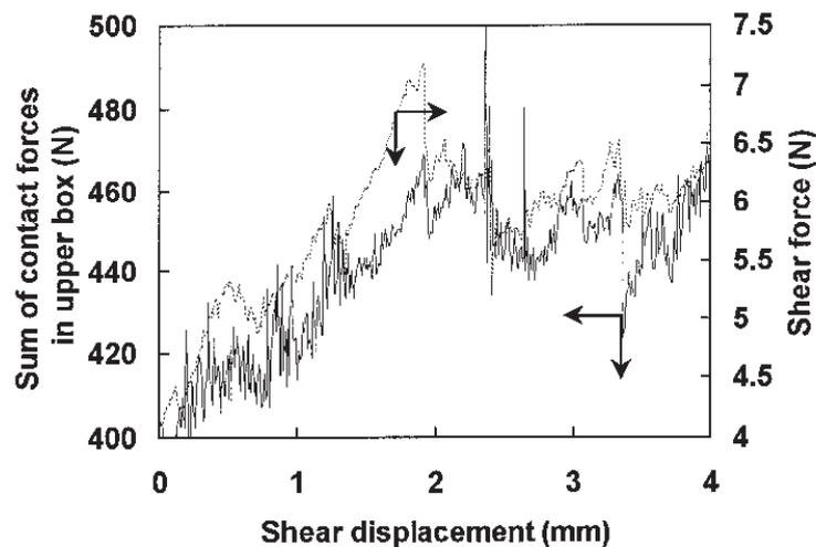
Fig. 9. Sum of contact forces in the upper box and shear force.
