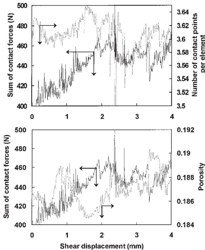
Fig. 8. Relationship between the sum of contact forces and Interlocking in the upper box.
