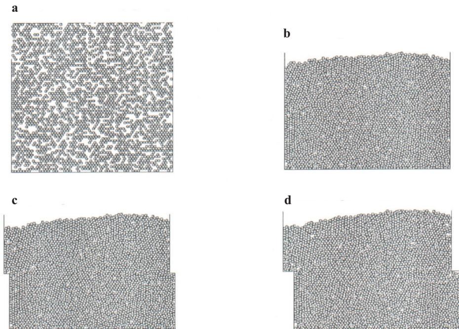
Fig. 3. Snapshots of the simulation results: before consolidation by gravity force (a), shear displacement : 0 mm (b), 2 mm (c), and 4 mm (d).
