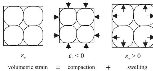
Fig. 1. Illustration of volumetric strain resulting from compaction by confining pressure and kernel swelling.
