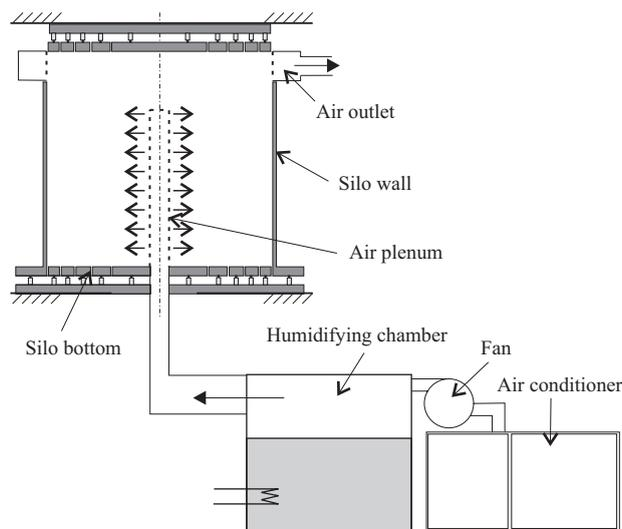
Fig. 3. Model silo with wetting equipment.
