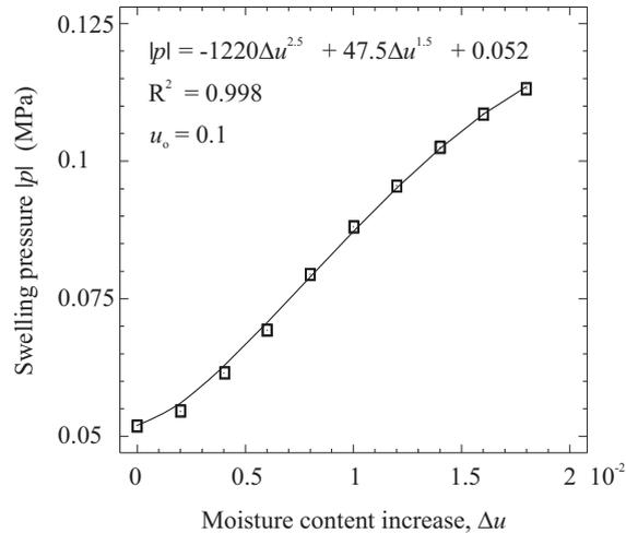
Fig. 2. Approximation of the initial part of the swelling pressure - moisture content increase relation [6].
