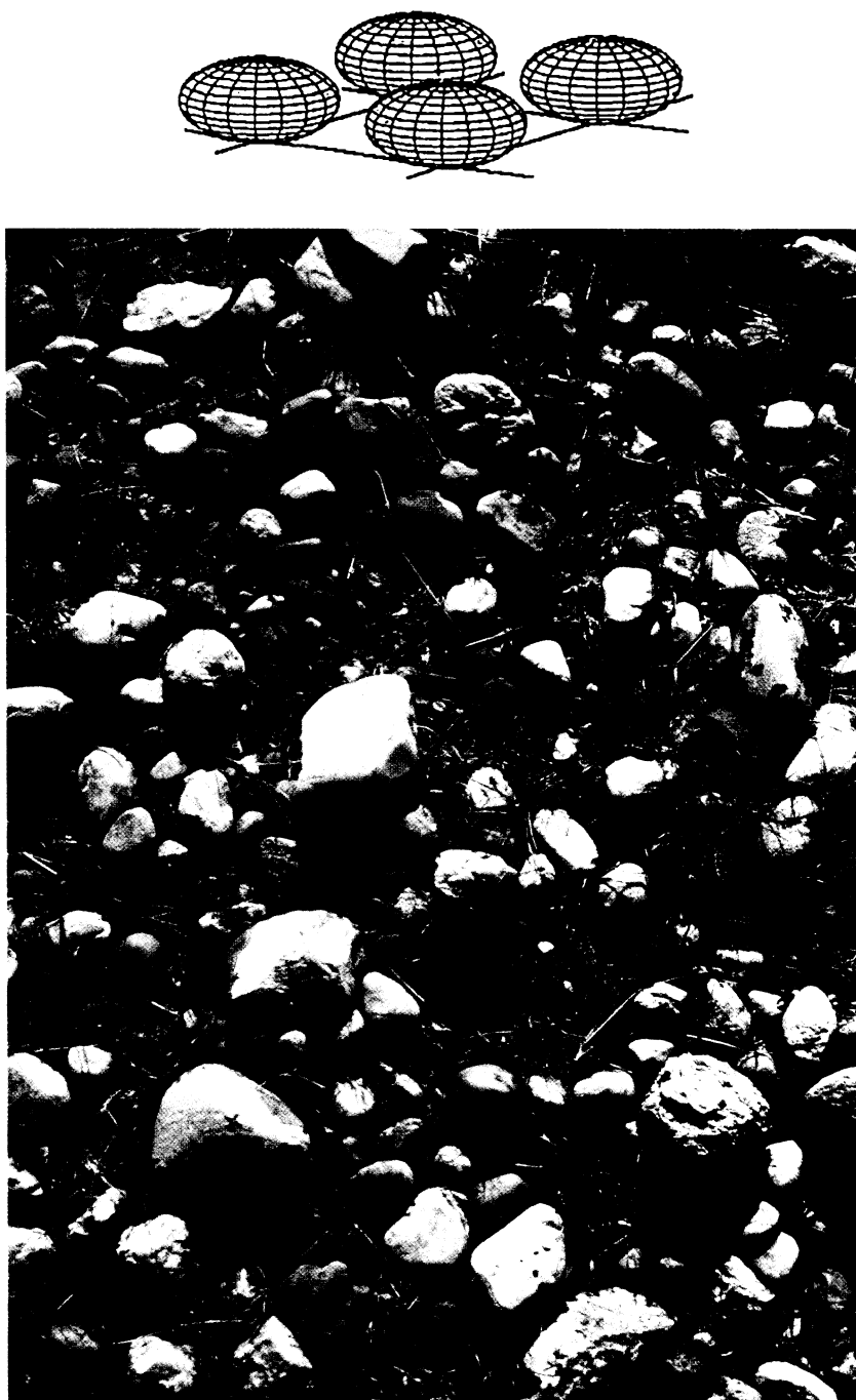
Fig. 2. Photography of the tested soil surface and the geometrical structure, being the result of the geometrical model inversion, used in the paper.
