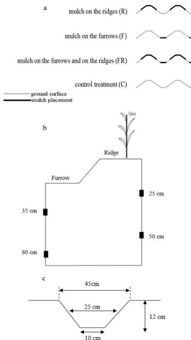
Fig. 1. Schematic view of the different mulch treatments (a), location of the maize crop and soil sampling for the control treatment (b) and experimental furrow cross-section (c).
