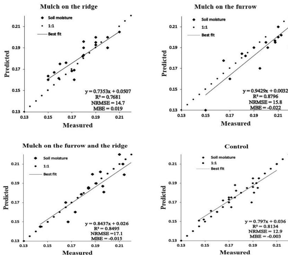
Fig. 7. Observed and simulated (HYDRUS-2D) soil water content ( $\text{cm}^3 \text{cm}^{-3}$ ) for each treatment.
