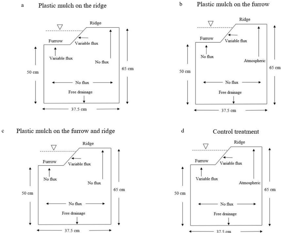
**Fig. 3.** Schematic view of the boundary condition related to the plastic mulch on the ridge (a), plastic mulch on the furrow (b), plastic mulch on the ridge and the furrow (c) and the control (d) treatments defined in HYDRUS-2D model.
