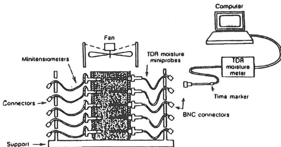
Fig. 2. Structural setup of the experimental stand. A soil core under investigation is kept in a metal sampling cylinder. An array of five minitensiometers and another array of five TDR soil moisture miniprobes are installed, marking of five independently monitored layers of the soil. Spiral arrangement of the probes is not visualized.
