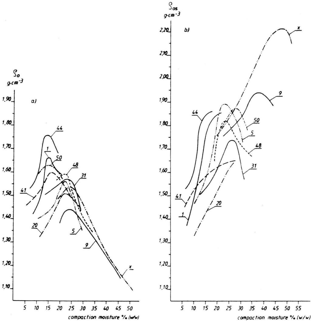
Fig. 3. Dependence of bulk density on consolidating moisture and shrinkage of soil aggregates: a) after consolidation, b) after shrinkage.
