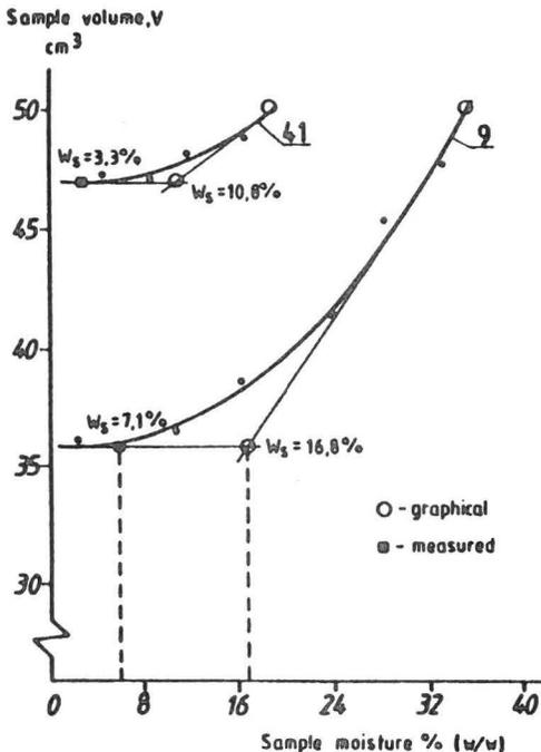
Fig. 2. Graphical appointed and measured value of soil shrinkage limit.
