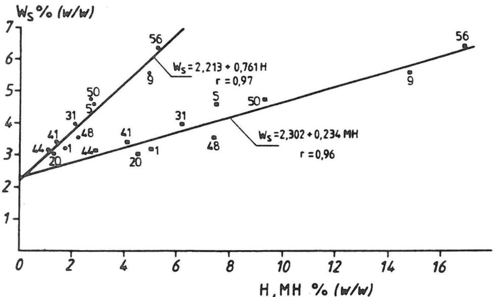
Fig. 5. Relationship between moisture at shrinkage-limit ( $W_s$ ) and hygroscopic water ( $H$ ) as well as maximal hygroscopic water ( $MH$ ).
