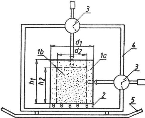
Fig. 1. Scheme of device for measurement of soil shrinkage: 1a- soil sample before shrinkage, 1b- soil sample after shrinkage, 2- perforated plate, 3- measuring sensors, 4- stand, 5- scale pan.
