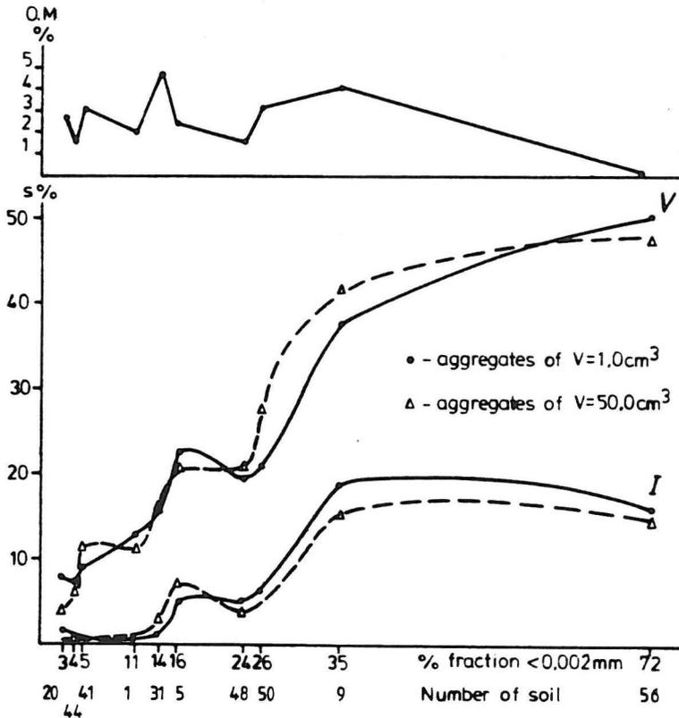
**Fig. 4.** Dependence of weak and strong consolidated soil aggregates on clay and organic matter content.
