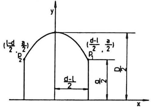
Fig. 2. The parabola describing a cross section of the lateral surface area.
