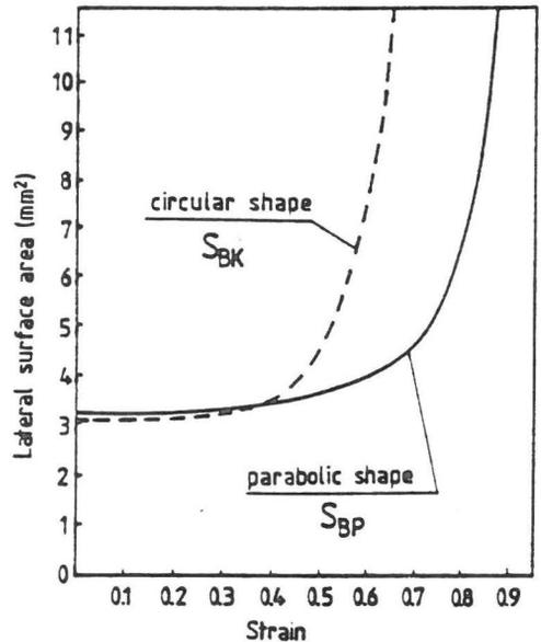
Fig. 3. A lateral surface area of barrel for parabolic shape  $S_{BP}$  and for circular shape  $S_{BK}$  related to strain of convex body during compression between parallel plates.
