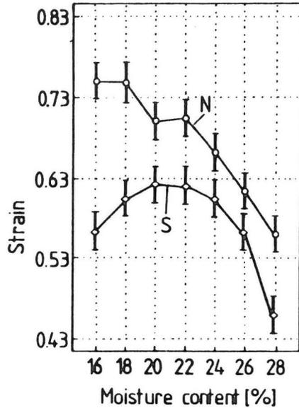
Fig. 4. Strain noticed at the break of seed shell for pea of Nike (N) and Sześciotygodniowy (S) varieties compressed between parallel plates at different moisture level.
