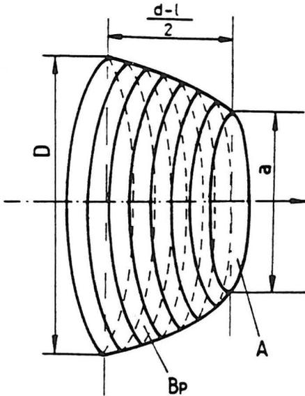
Fig. 1. The surface area of bottom  $A$  formed as the effect of flattening and the lateral surface area of the barrel  $B_p$  created by rotation of a curve around axis  $x$ .
