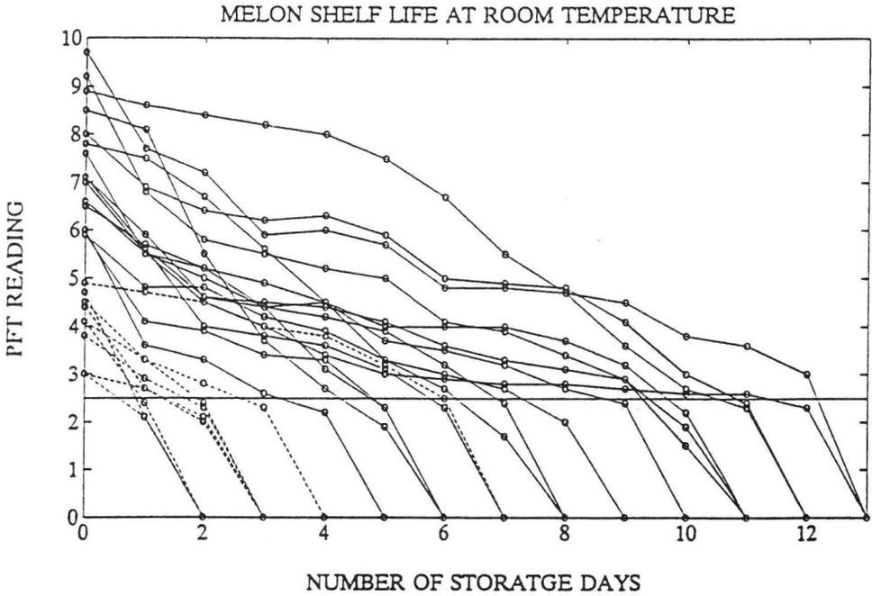
Fig. 4. Reduction of melon firmness with time, as indicated by consecutive *PFT* measurements every two days, on a sample of 25 melons stored at room temperature. The horizontal line of *PFT*=2.5 was chosen arbitrary, as a cut off firmness level which indicates the end of the useful shelf-life of these melons. The thick solid line denotes the mean firmness reduction of the entire melon sample with time.
