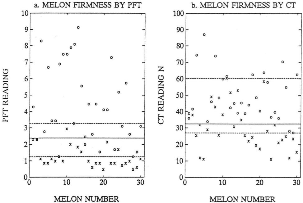
Fig. 3. Scattergrams of *PFT* readings (a) and *CT* readings (b), on a sample of 30 'soft' (x) melons and 30 'firm' (o) melons.
