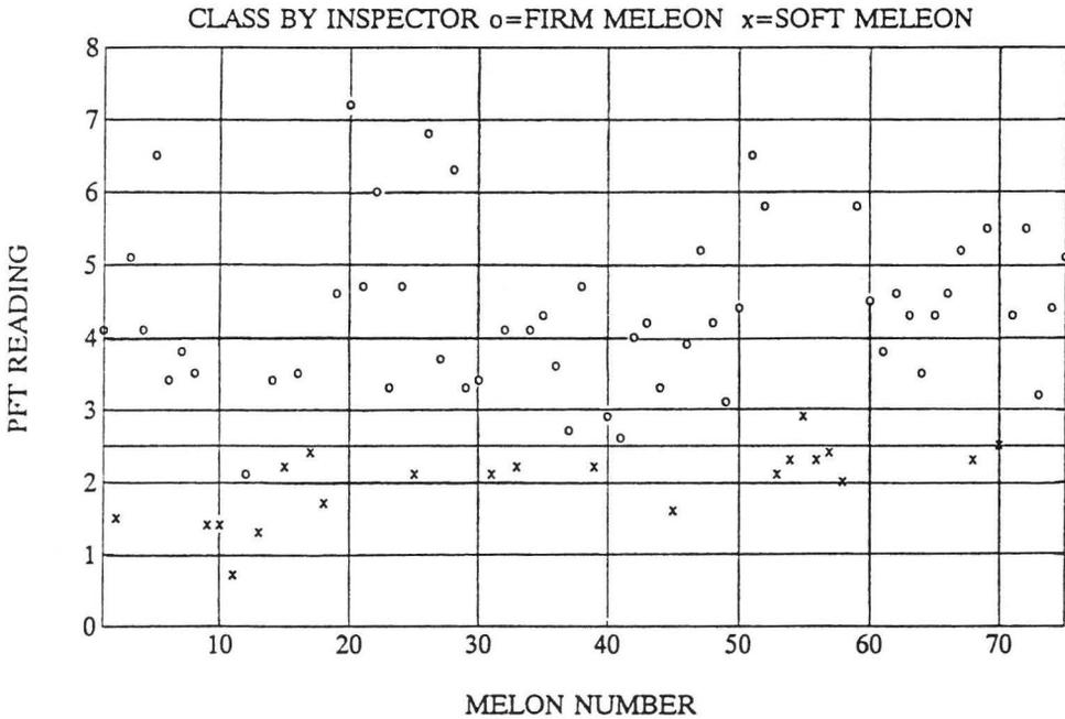
Fig. 5. Typical example of results obtained at a commercial quality inspection station wherein *PFT* readings on a sample of 75 melons are plotted, while those classified as 'firm' and 'soft' by sensory hand squeezing are marked by o's and x's, respectively.
