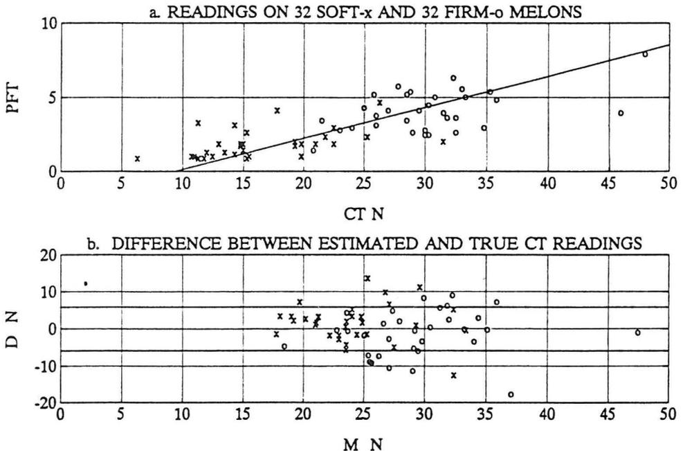
Fig. 2. (a) Scattergram of *CT* versus *PFT* readings on a sample of 64 'firm' (o) and 'soft' (x) melons. (b) Distributions of differences between estimated and true *CT* readings on the melon sample of Fig. 2a after translation from *PFT* to  $PFT_{ct}$  by the scale translation line represented by Eq. (2).
