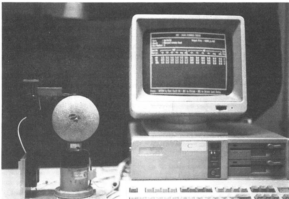
Fig. 1. Non-destructive fruit firmness measurement system, showing sensor and microcomputer. In operation, one side of the fruit is placed on the head of the vibrator and the sensor finger is lowered onto its other side, as shown. A firmness reading is then automatically recorded by the microcomputer.
