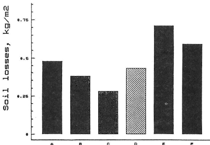
Fig. 2. Erodibility of loess soil based on laboratory studies with the rainfall simulator. A - non-eroded, B - slightly eroded, C - moderately eroded, D - severely eroded, E - completely eroded, F - deluvial soil.
