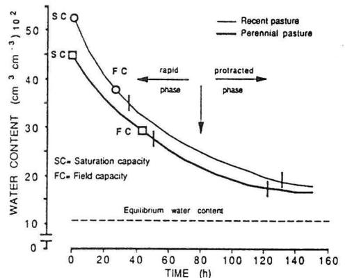
Fig. 3. Changes in water content versus time, of undisturbed soil samples from recent pastures given two year grazing (RPG) and from perennial pastures long-term grazed (PPG).
