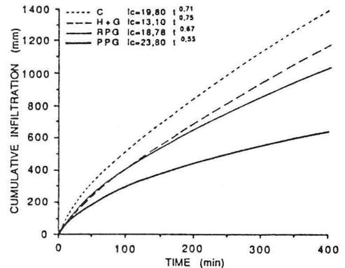
Fig. 2. Water cumulative infiltration in soils of recent pastures given two year grazing (RPG) or haymaking plus grazing (H+G), of the control plots (C), and of those from perennial pastures long-term grazed (PPG).
