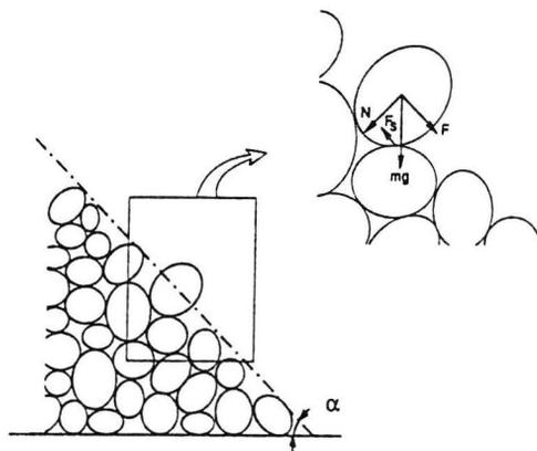
Fig. 5. A particle sliding down on the surface of a heap of granular material. The relatively rough surface results in supportive forces ( $F_s$ ) that interfere with gravitational force.
