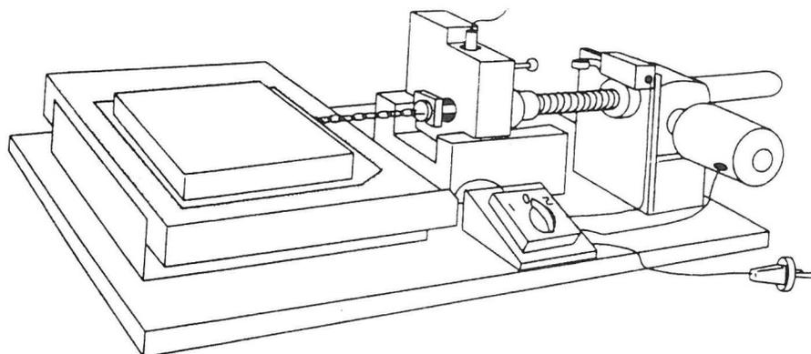
Fig. 4. View of equipment used for determining internal and external dynamic friction.
