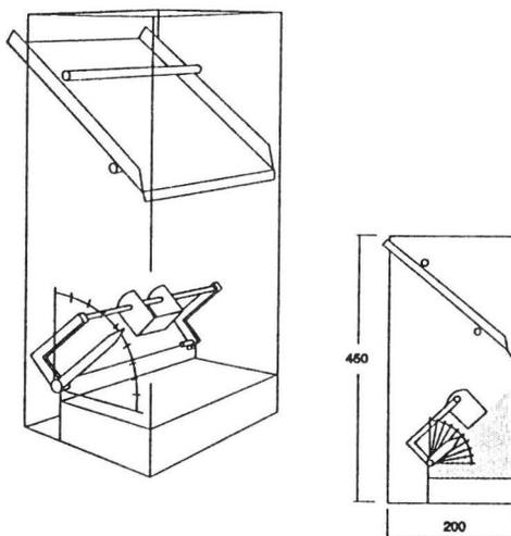
Fig. 3. Equipment used for determining dynamic angle of repose. Scales are in millimeters.
