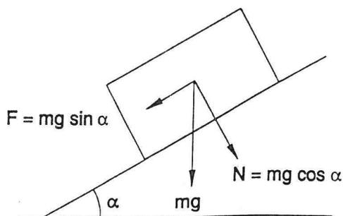
Fig. 1. A body on a sloping surface. The weight is divided into perpendicular components.
