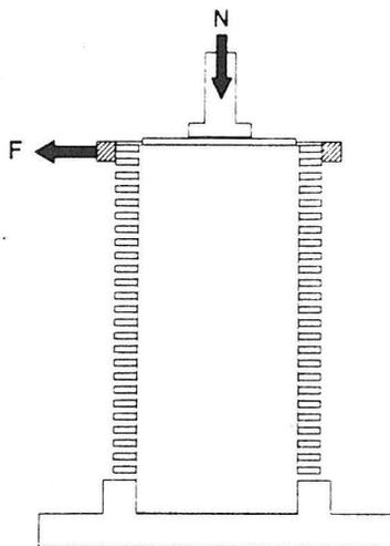
Fig. 2. Schematic view of apparatus for determining internal static friction.
